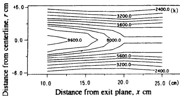
Fig. 11 Two-dimensional distribution of the translational temperature of the argon neutral atoms. Input power 1.8 kW, propellant flow rate 0.24 g/s.
