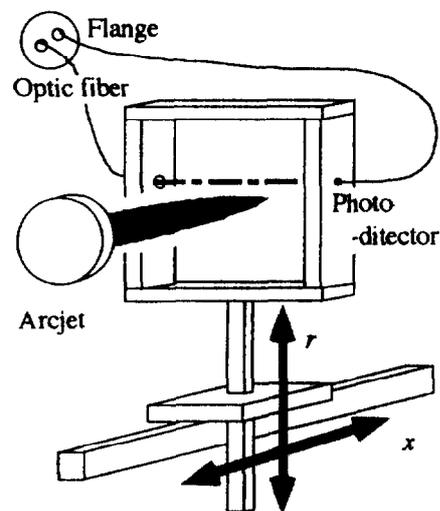
Fig. 3 Optic arrangement mounted on a two-dimensional traverse system.
