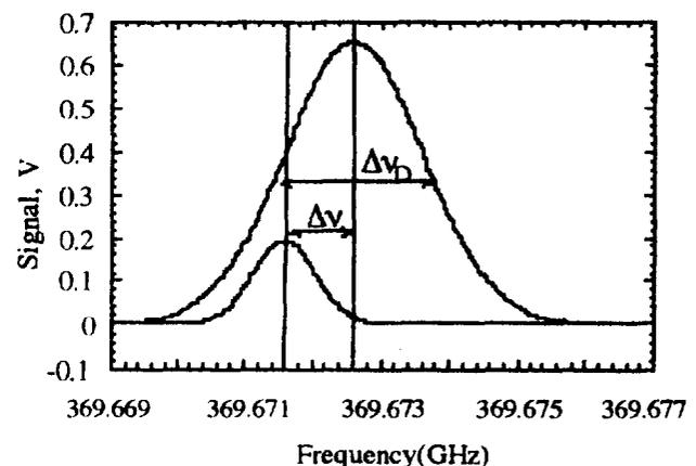
Fig. 6 Absorption profile of the transmitted lasers through the arcjet plume (upper) and the argon discharge tube (lower).
