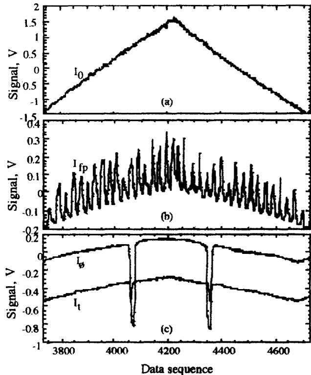
Fig. 5 Typical records. (a) temporal variation of incident laser intensity. (b) Fabry-Perot etalon signal, (c) transmission profile of the oblique probe laser beam (upper) and the one through the argon discharge tube (lower).
