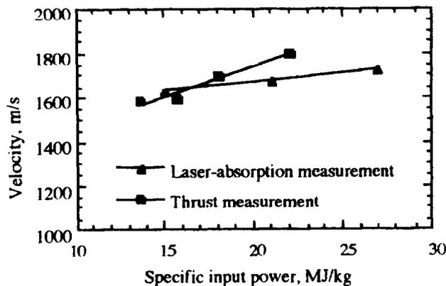
Fig. 8 Measured local velocity with the mean flow velocity derived from thrust measurements. Propellant mass flow rate is 0.12 g/s.
