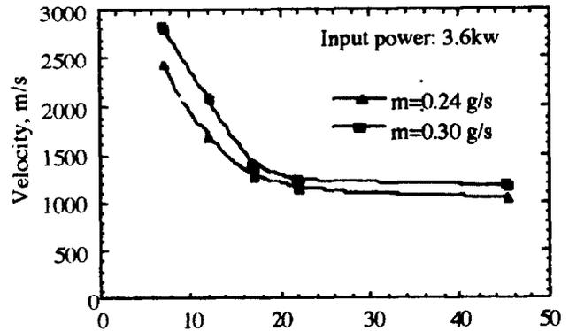
Fig. 9 Distributions of the velocity along the thruster centerline.
