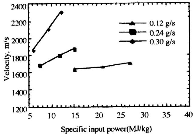
Fig. 7 Plume velocity vs. specific input power measured at 7.0 cm downstream of the nozzle exit plane.
