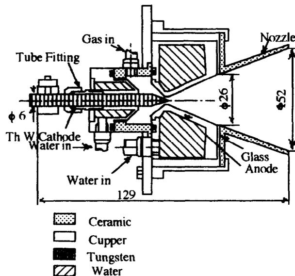
Fig. 1 A cross section view of the arcjet thruster
