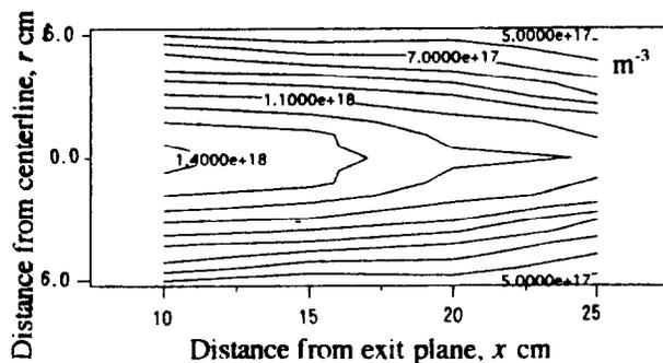
Fig. 12 Two-dimensional distribution of the number density of the argon neutral atoms. Input power 1.8 kW, propellant flow rate 0.24 g/s.
