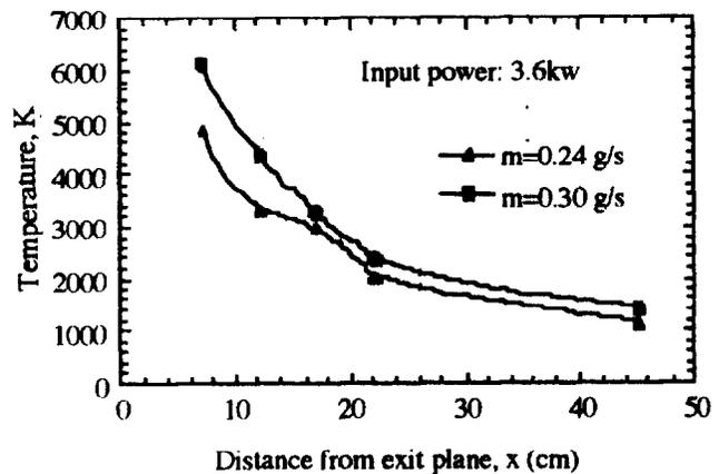
Fig. 10 Distributions of the temperature along the thruster centerline.
