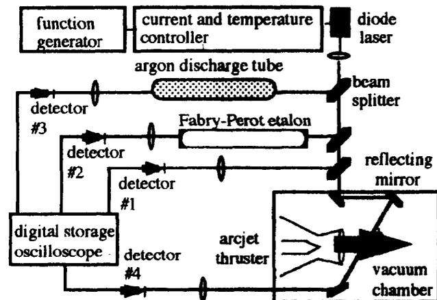
Fig. 2 Schematic of the diode laser absorption spectroscopy system.
