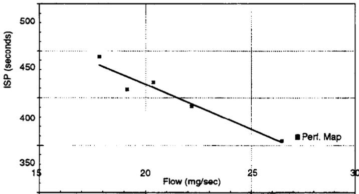
Figure 5. Specific impulse versus flow rate
