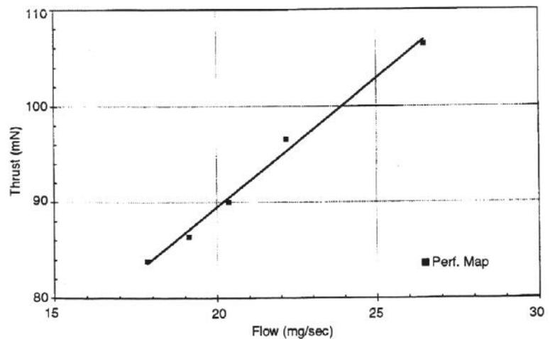
Figure 4. Thrust versus flow rate
