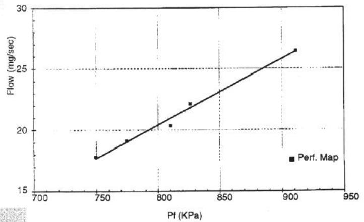
Figure 3. Flow rate versus feed pressure
