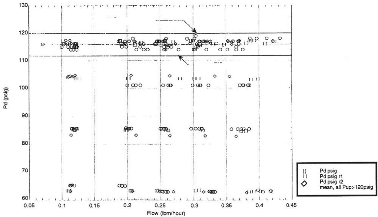
Figure 13. Liquid regulator characteristic
