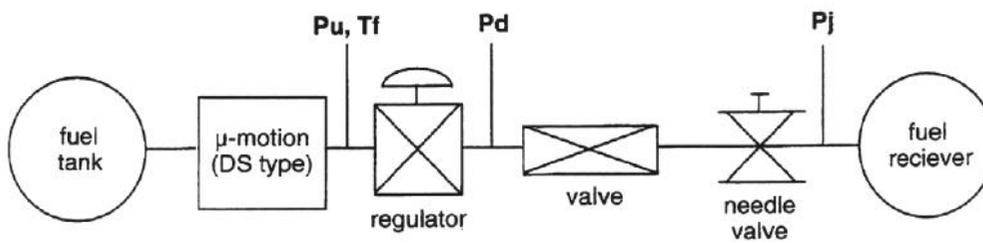
Figure 12. Regulator test setup
