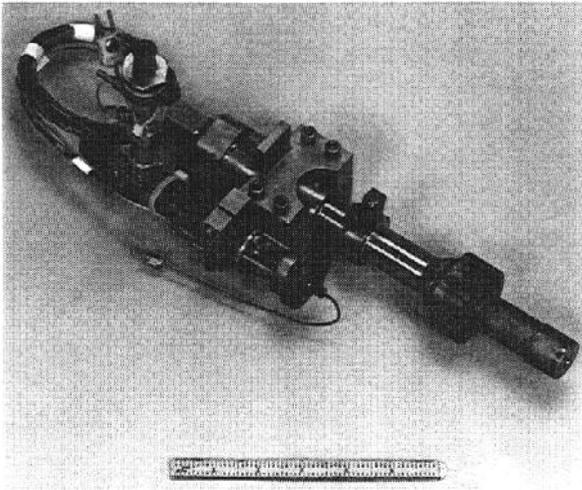
Figure 1. Arcjet thruster test article.
