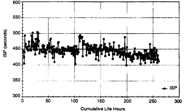
Figure 8. Specific impulse characteristics
