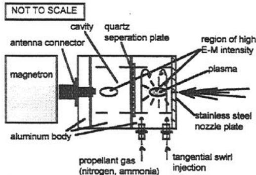
Fig. 3: Engine Schematic.
