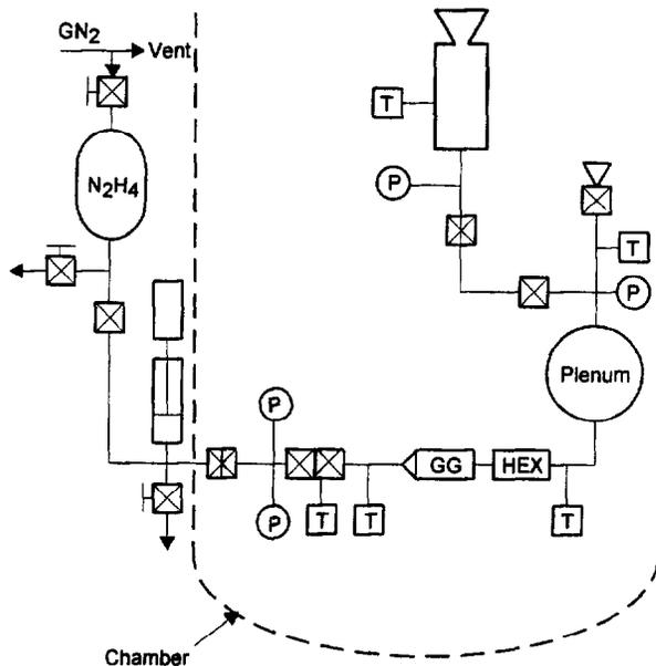
Figure 3.0. Laboratory PPG System/Arcjet Test Setup
