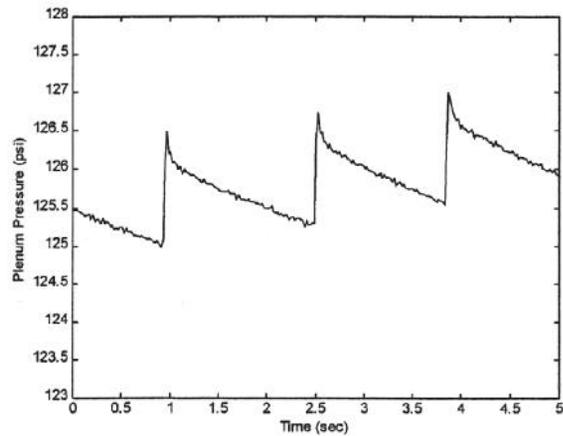
Figure 8.0 Plenum Pressure Response
