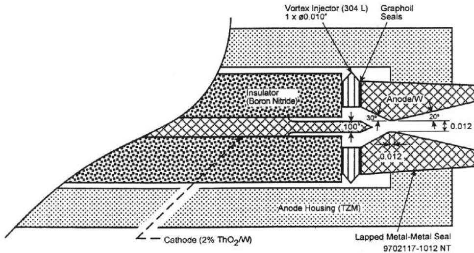
Figure 6.0. Modified NASA LeRC 500W Arcjet
