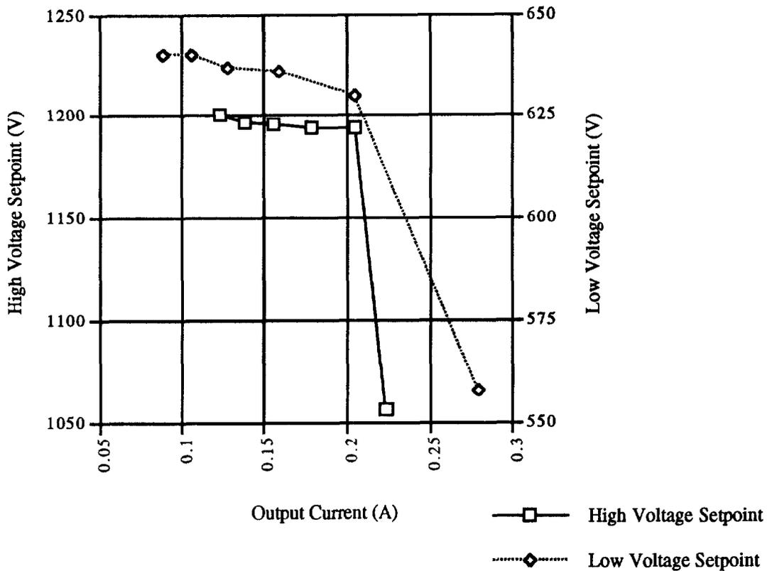
Figure 6. Beam supply load regulation test results
