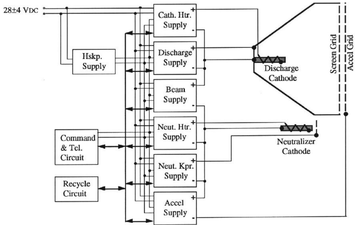
Figure 1. Low power ion propulsion system block diagram
