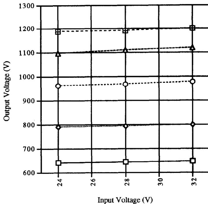
Figure 5. Beam supply line regulation test results
