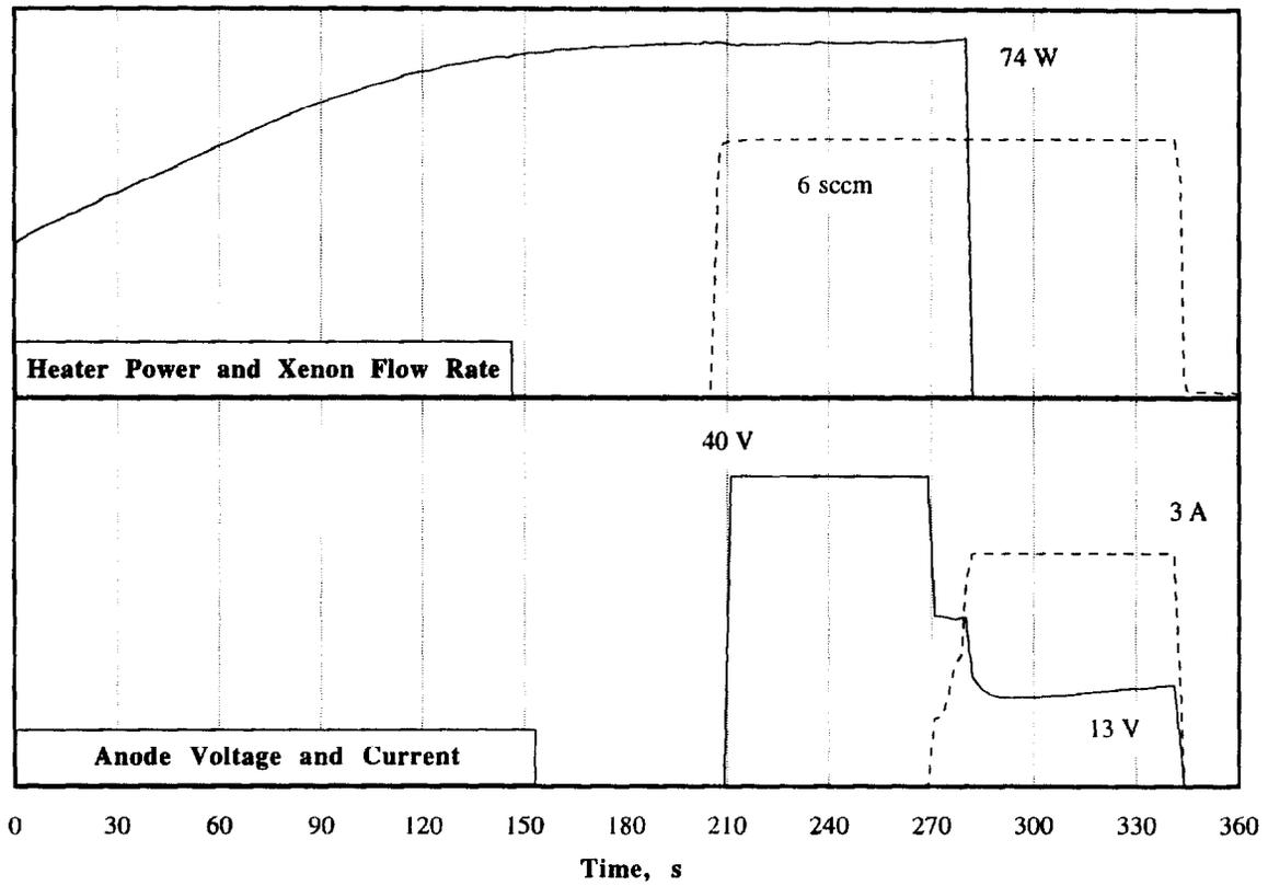
Figure 3 - Typical HCA ignition cycle data.
