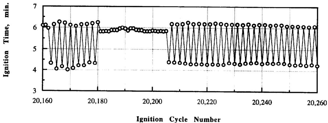
**Figure 7 - An example of oscillating ignition times.**
