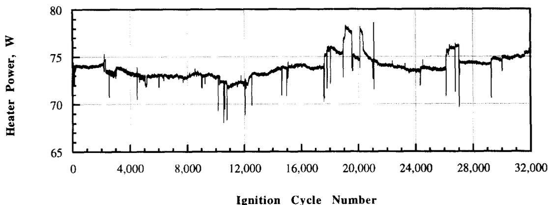
Figure 10 - Heater input power versus ignition cycle. The maximum heater power each cycle is depicted.
