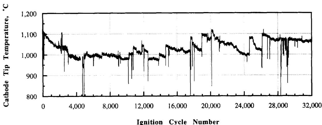
Figure 9 - Cathode tip temperature versus ignition cycle. The temperature is recorded 3.5 minutes after the heater power is applied each cycle.
