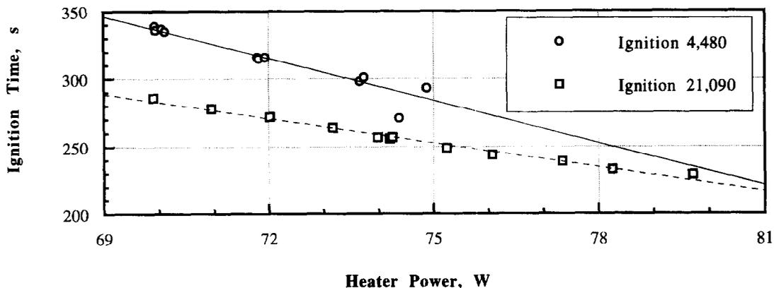
Figure 8 - Heater power versus ignition time.
