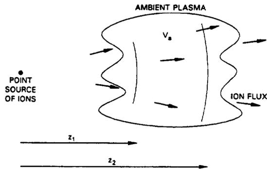
Fig. 3 Scattering Model of Ion Flux Loss due to Collisions downstream of Hollow Cathodes
