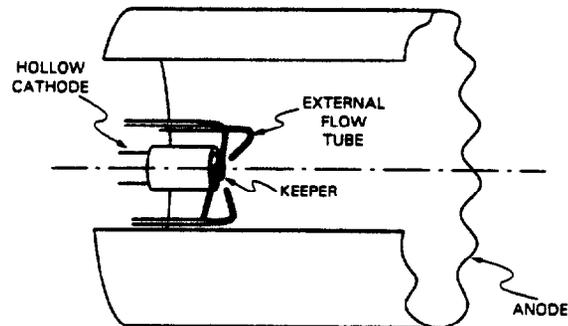
Fig. 2 Setup for External-Expellant-Flow Experiment
