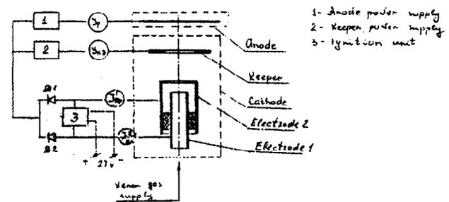
Fig. 8 Heaterless cathode power supply and flow arrangement
