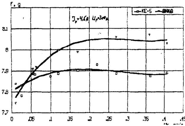
Fig.14 SPT-100 thrust relationship to the cathode flow
