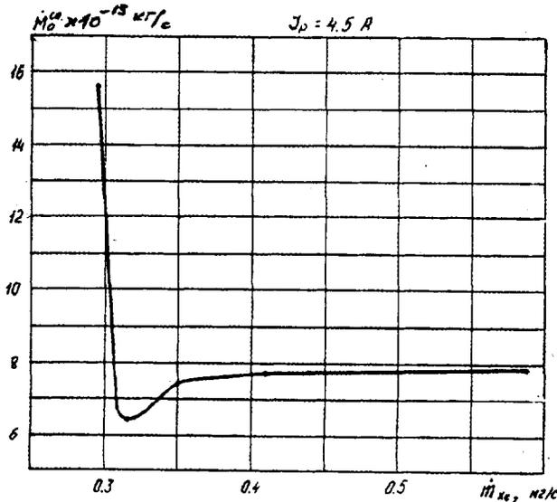
Fig.4 Doping material erosion rate vs cathode flow rate
