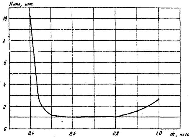
Fig.5 Number of ignition impulses for cathode to switch on vs cathode flow rate
