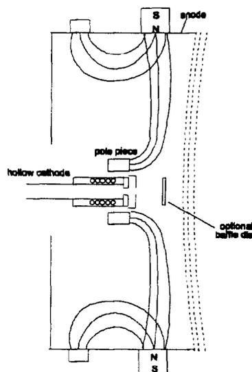
**Figure 2. Schematic diagram of gridded ion engine which reduces residence time.  $C_{60}$  sublimator and full magnetic field circuit not shown.**
