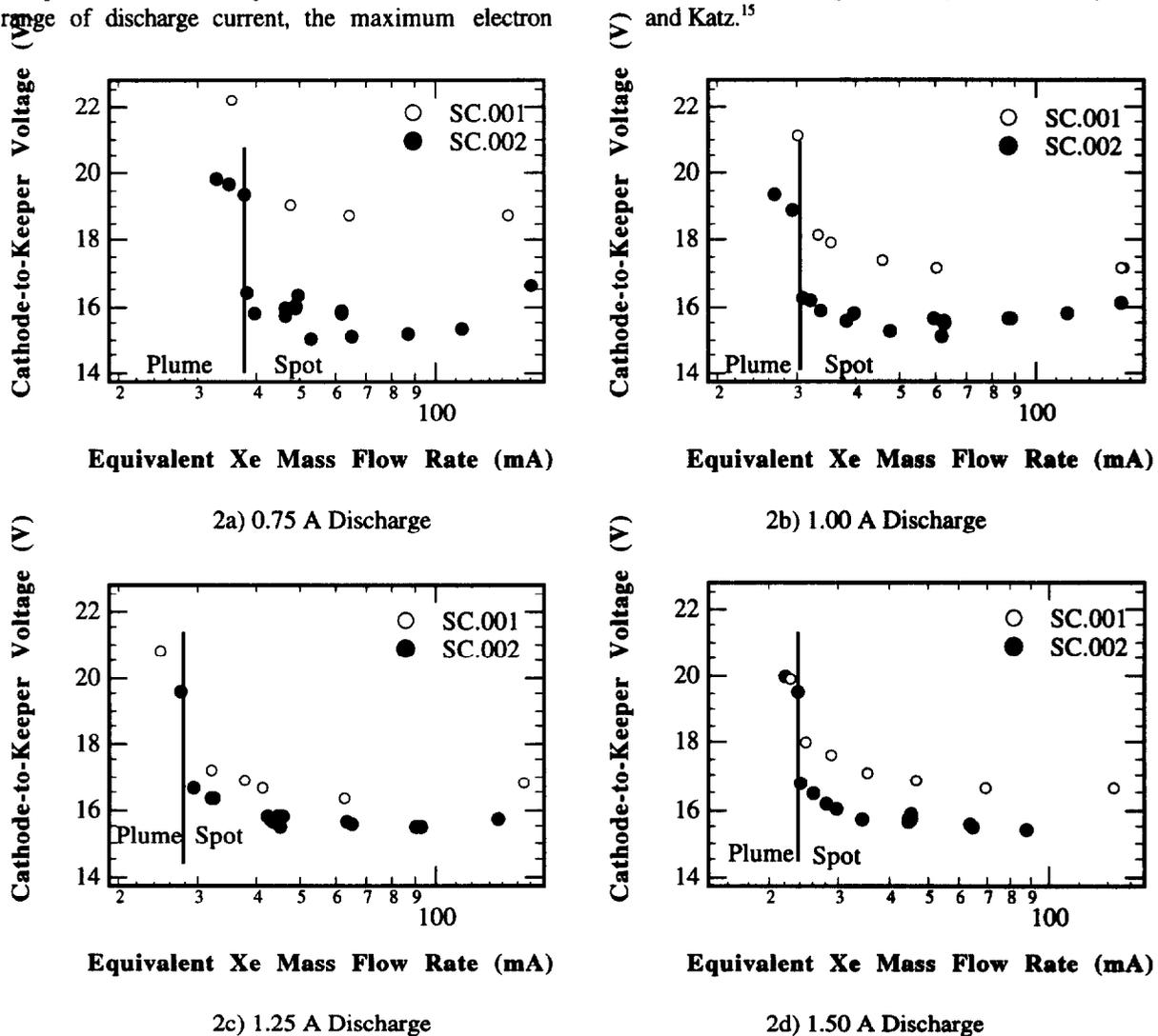
Fig. 2 - Performance Characteristics of the Cathodes with Impregnated Porous Tungsten Inserts.
