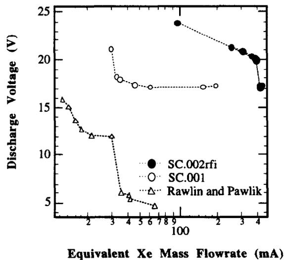
Fig. 3 - Comparison of Xe Cathodes at 1 A with Two Different Insert Geometries and a Hg Cathode at 0.45 A from Rawlin and Pawlik.<sup>7</sup>
