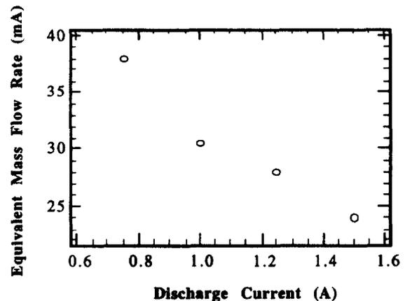
Fig. 4 - Flow rates Required to Maintain Spot-Mode Emission.
