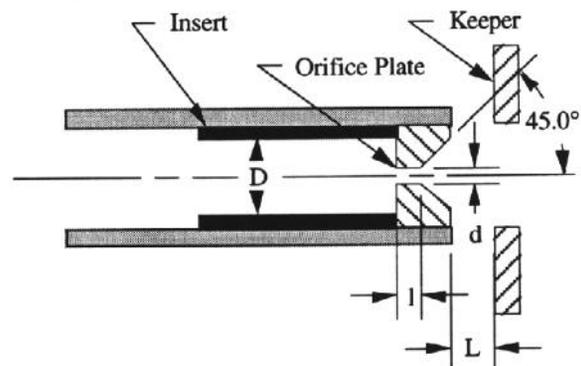
Fig. 1 - Schematic of the Hollow Cathode Experiments.
