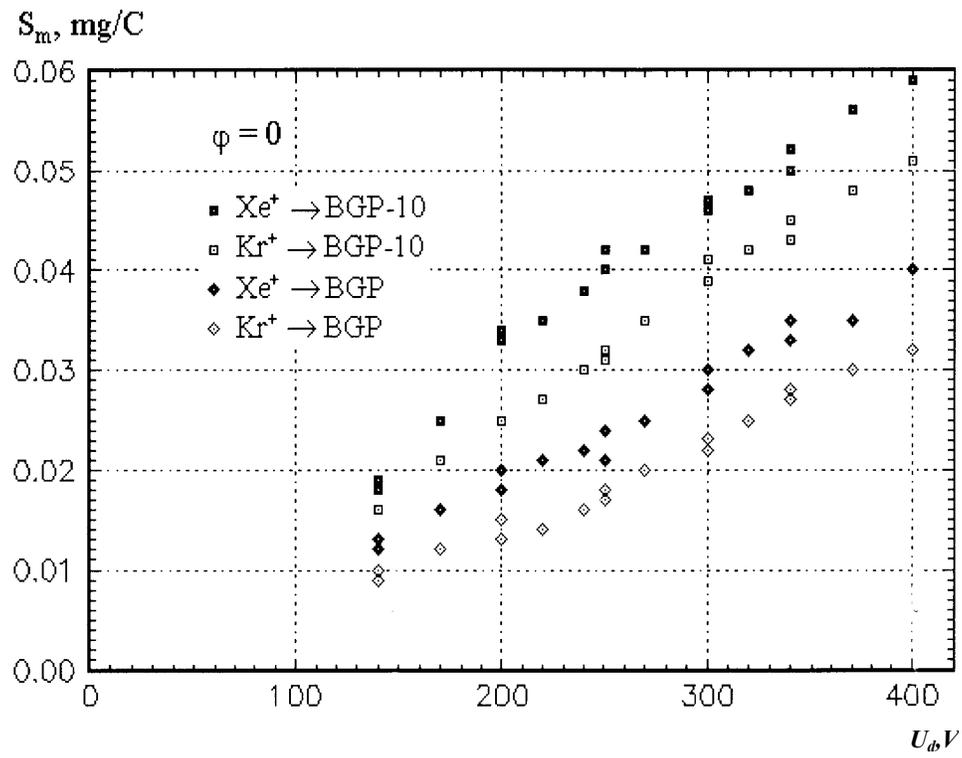
Figure 5 - The sputtering yield dependence on discharge voltages (ion energy).
