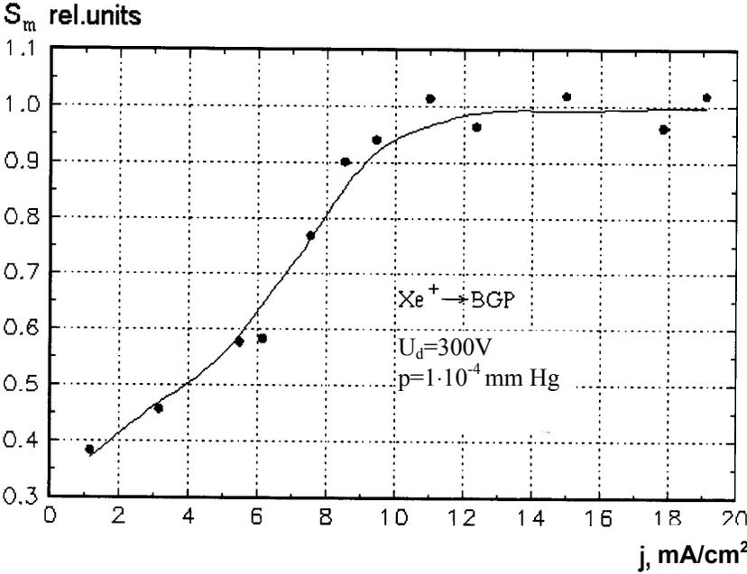
Figure 3 - The sputtering yield dependence on ion current density.
