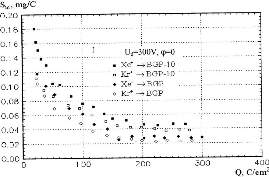
Figure 4 - The sputtering yield dependence on the type ion charge Q.
