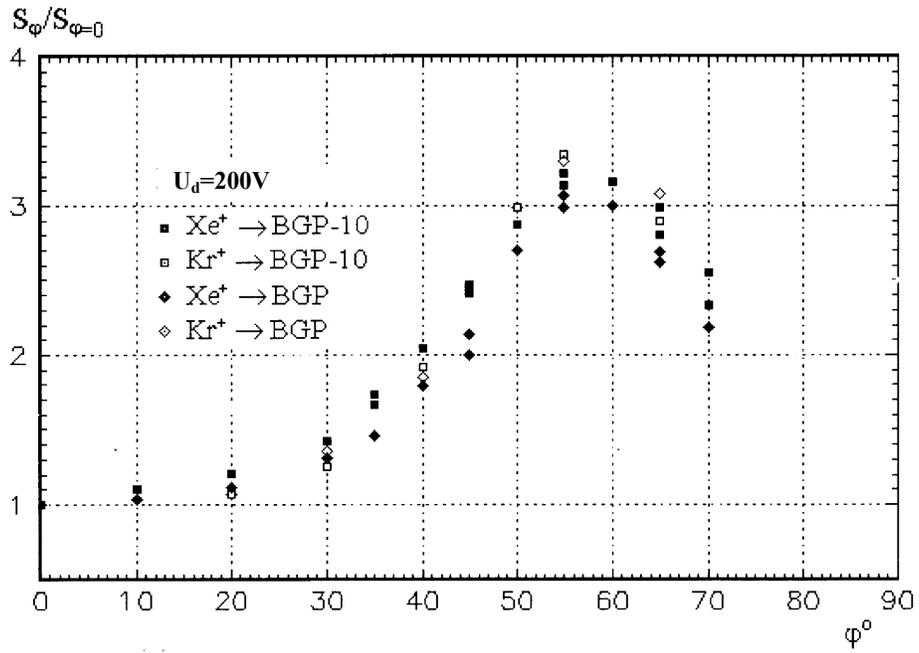
Figure 6 - The sputtering yield dependence on the incident angle.
