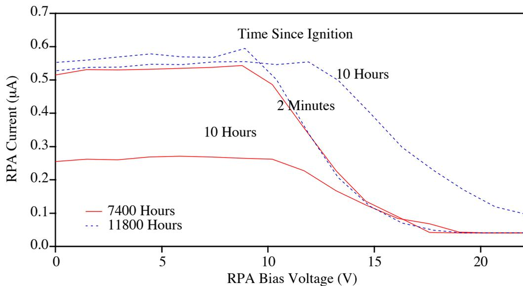
Figure 21: Ion energy distributions measured with the retarding potential analyzer.
