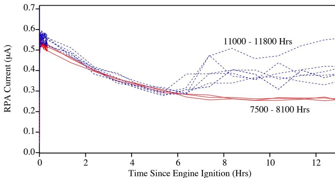
Figure 20: Total ion current collected by the retarding potential analyzer as a function of time after engine ignition.
