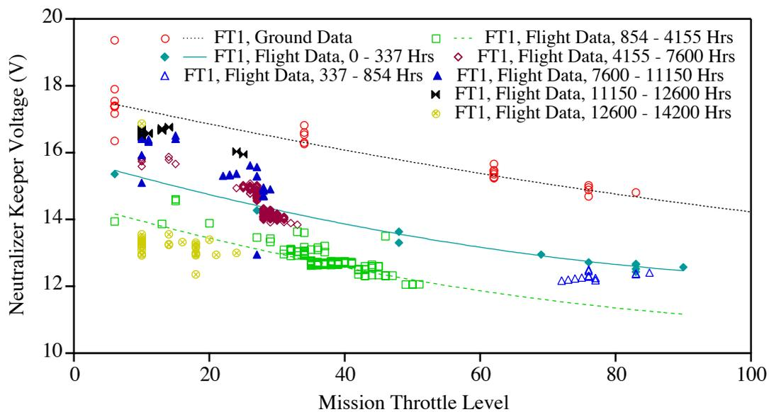
Figure 19: Neutralizer keeper voltage measured in space and in ground tests.
