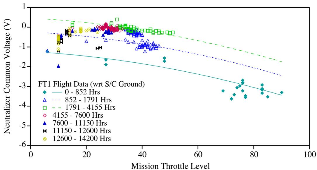
Figure 22: Neutralizer common voltage measured with respect to spacecraft ground in space.
