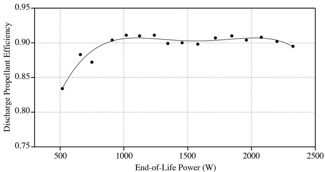
Figure 2: NSTAR ion thruster discharge propellant utilization efficiency.
