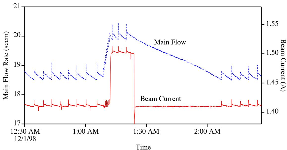
Figure 13: Example of throttle-up and throttle-down sequences.
