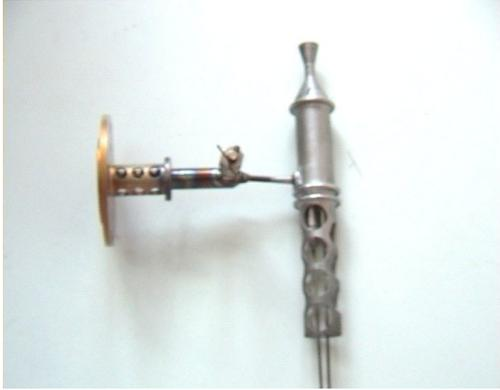
Fig. 1 The picture of resistojet
