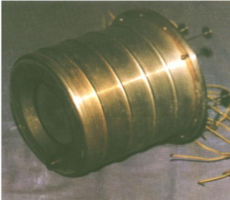
Fig.8 The picture of Xenon ion thruster
