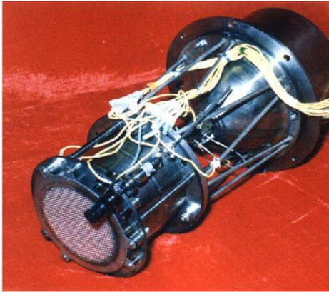
Fig. 7 The picture of Mercury ion thruster
