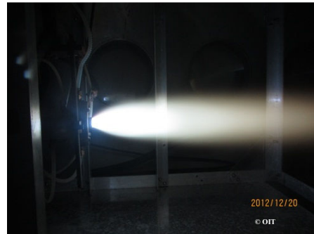
Figure 13. DC Arc jet Firing (N 2 @3.5 SLM+H 2 O)
