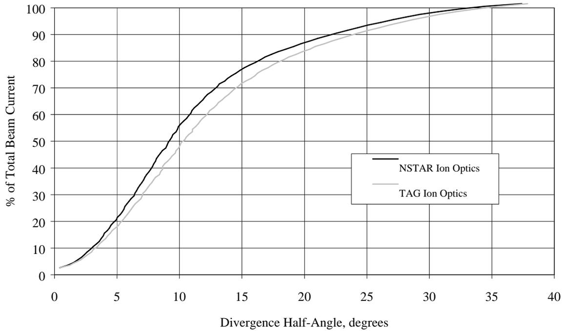
**Fig. 8. Percentage of total beam current enclosed in a given divergence half-angle for TAG and NSTAR ion optics at a THe19. Beam current densities for TAG ion optics were measured prior to ion optics burn-in.**
