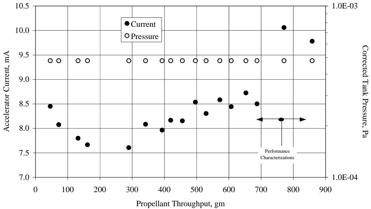
**Fig. 5. Accelerator current and corrected tank pressure as a function of propellant throughput for TAG ion optics at TH15.**
