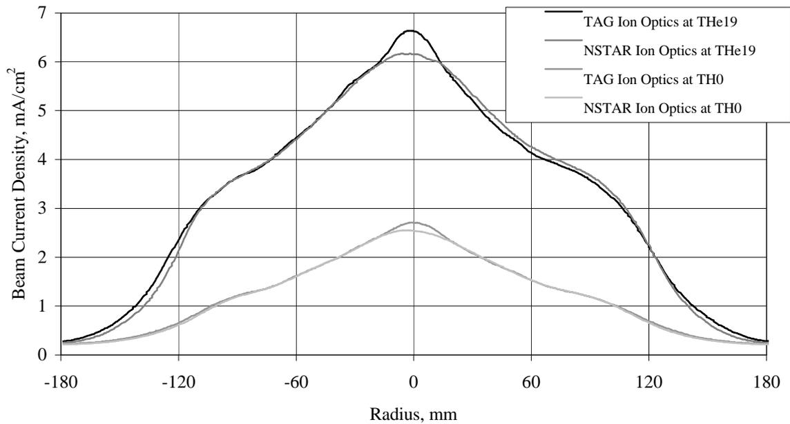
**Fig. 6. Radial beam current density profiles for TAG and NSTAR ion optics at THe19 and TH0. Beam current densities were measured 48-49 mm downstream of the ion optics' center. Beam current densities for TAG ion optics were measured prior to ion optics burn-in.**
