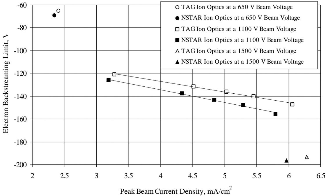
**Fig. 4. Electron backstreaming limit as a function of peak beam current density for TAG and NSTAR ion optics. Peak beam current densities were measured 48 mm downstream of the ion optics' center. Beam voltages here are power supply voltages.**
