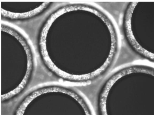
Fig. 8-6: Decel and Accel holes in the grid center
