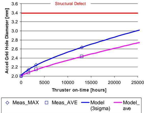
Fig. 8-3: Grid erosion data and prediction
