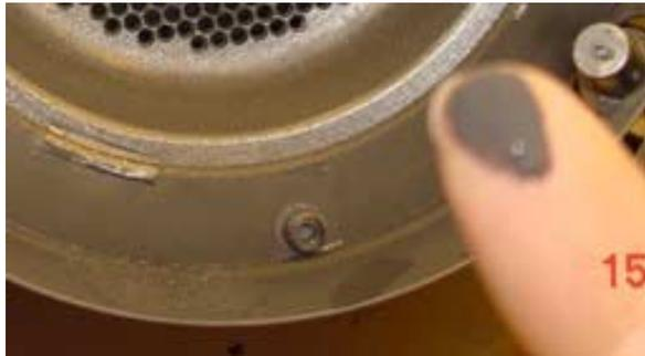
Fig. 9-2 Accumulation of graphite material in the thruster's sunshade
