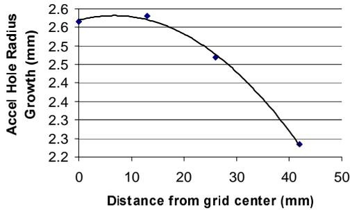
Fig. 8-2: Acceleration grid hole diameter as a function of the thruster radius
