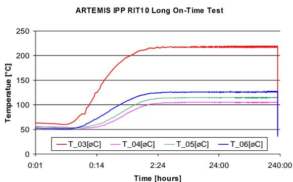
Fig. 12-1 RIT10 long duration test (219 hours) - logarithmic time scale -
