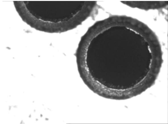
Fig. 8-7: Decel and Accel holes at the grid rim
