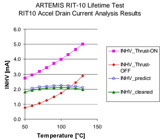
Fig. 9-4 Accel Drain Current Models
