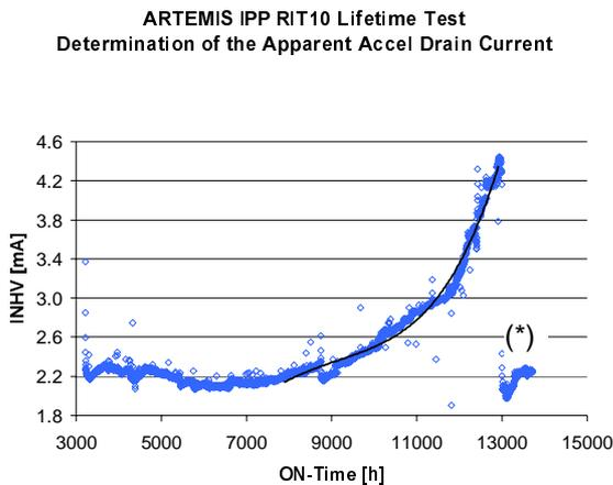
Fig. 9-5 Determination of the apparent accel drain current (black line)
