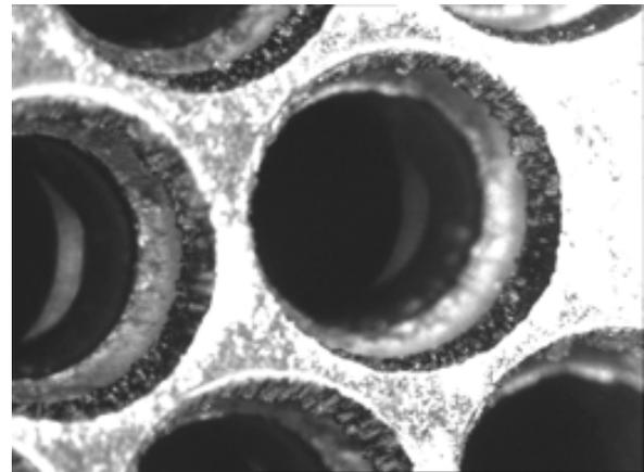
Fig. 8-1: Deceleration grid erosion close to the thruster rim
