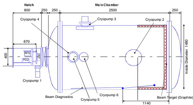
Fig. 6-1: Schematic of the ESTEC test chamber
