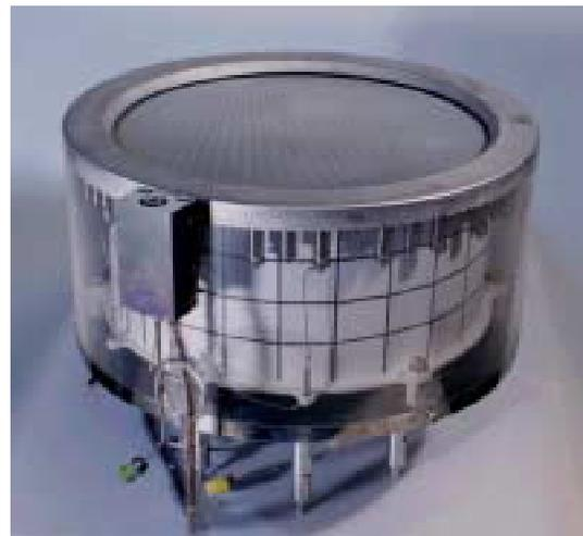
Figure 2 - Photograph of BBM-2 thruster.
