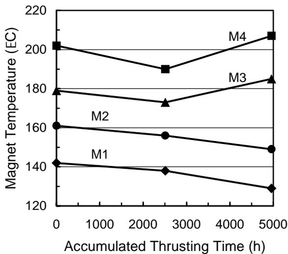
Figure 11 - Temperatures at discharge-chamber magnet rings.
