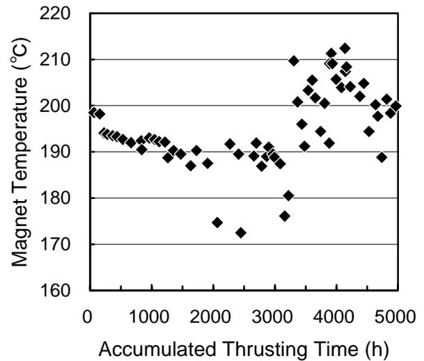
Figure 12 - Temperature variations of magnet ring M4.
