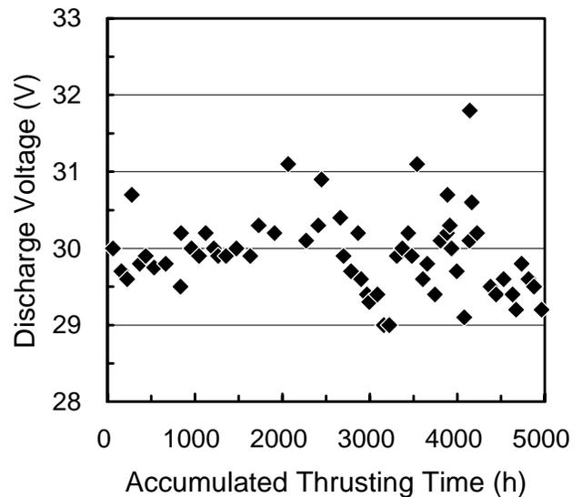
Figure 9 - Variations in discharge voltage.
