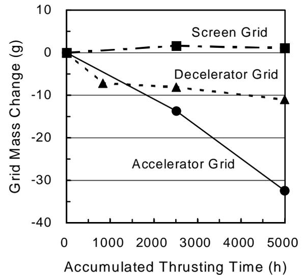
Figure 13 - Grid mass changes with time.
