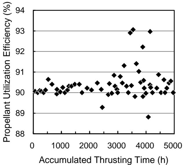
Figure 7 - Variations in discharge-chamber propellant utilization efficiency.
