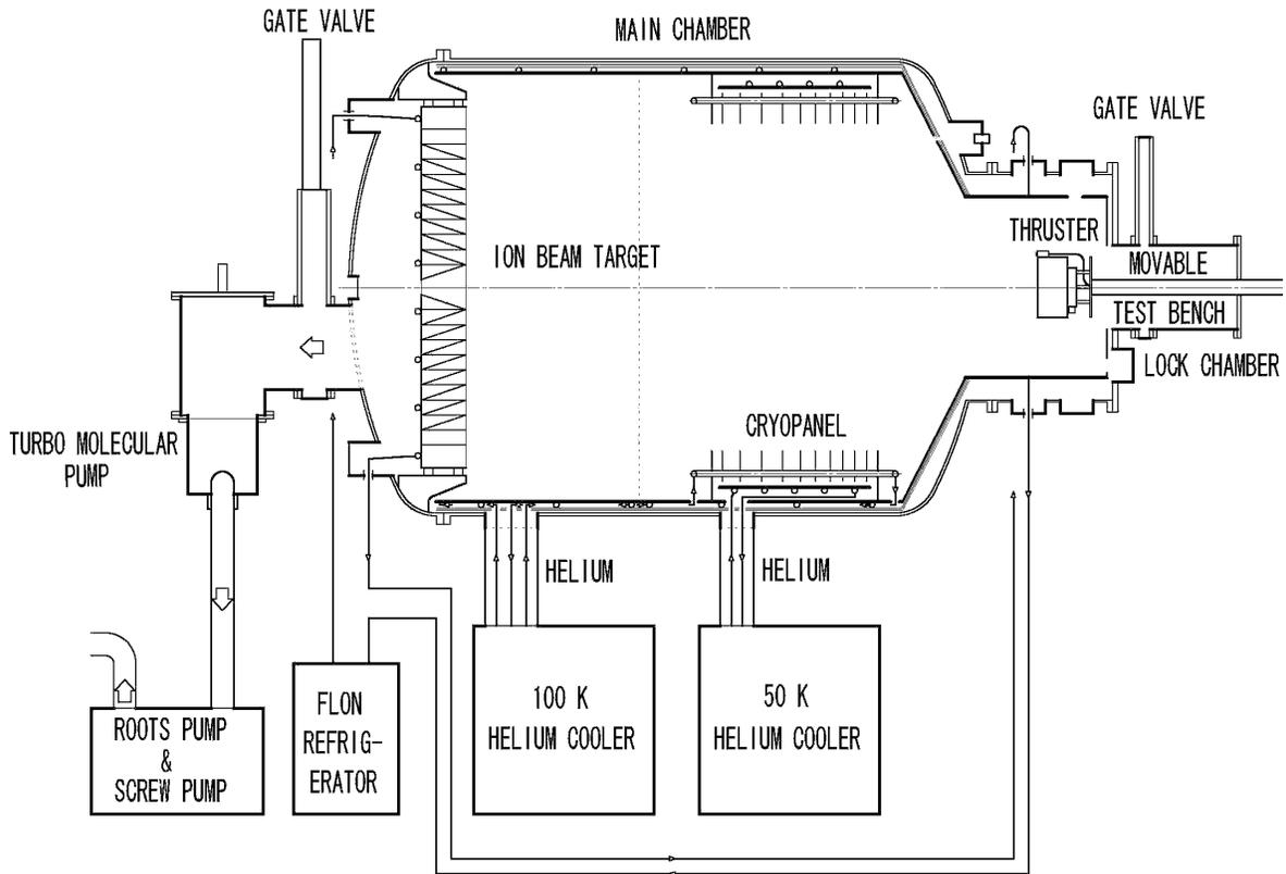
Figure 3 - Schematic view of test facility.
