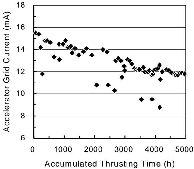
Figure 10 - Variations in accelerator grid current.
