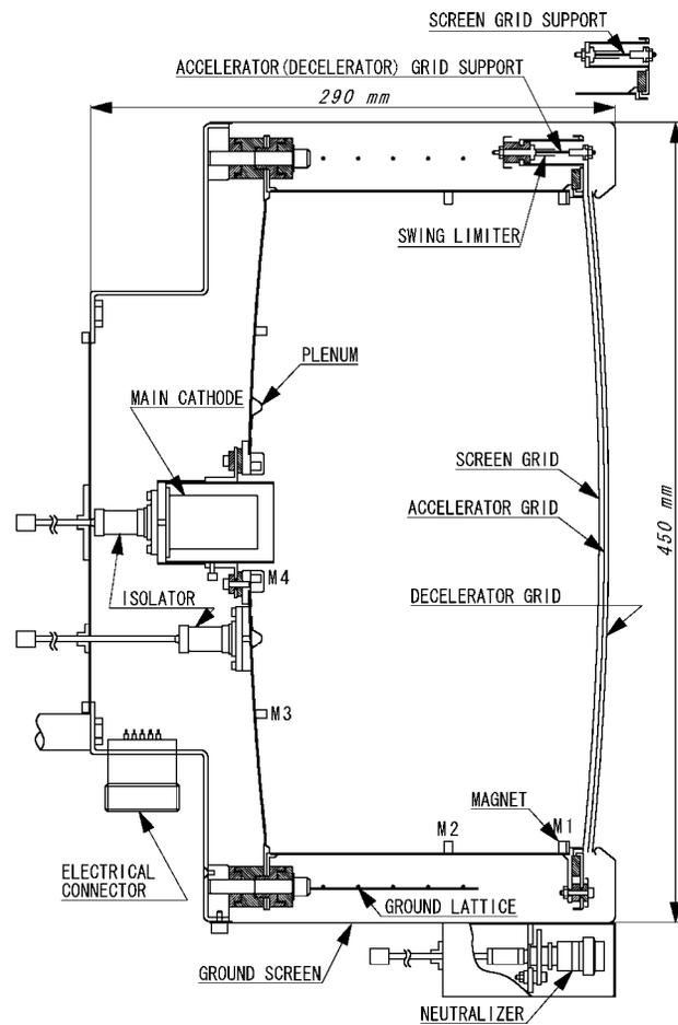
Figure 1 - Cross-sectional view of BBM-2 thruster.
