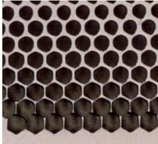
Figure 15 - Decelerator grid holes in periphery region.
