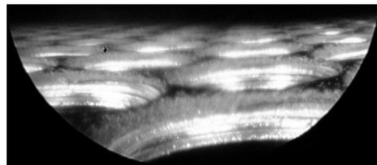
Figure 14 - Screen grid holes in center region.
