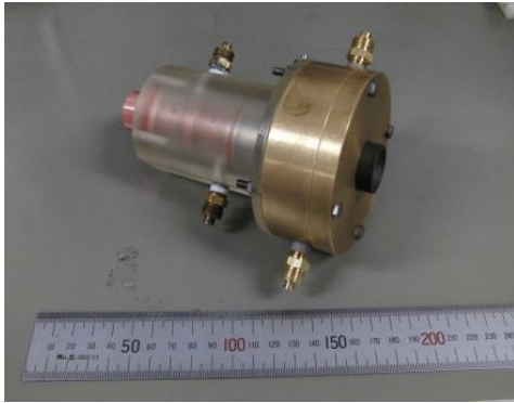
Figure 4. Photograph of low-power (1-3kW) direct-current arcjet thruster.
