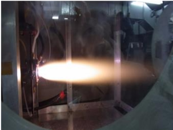
Figure 20. Photo of low-power arcjet plasma plume with HAN (SHP163) decomposed gas.
