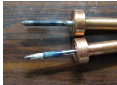
Figure 22. Photo of cathodes after operations with HAN (SHP163) decomposed gas.
