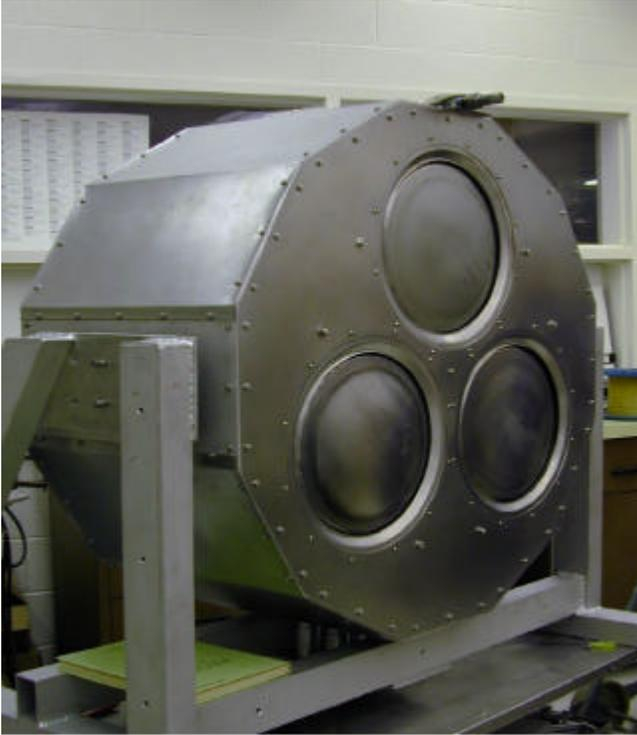
Figure 1 - High-power, 76-cm diameter ion thruster.
