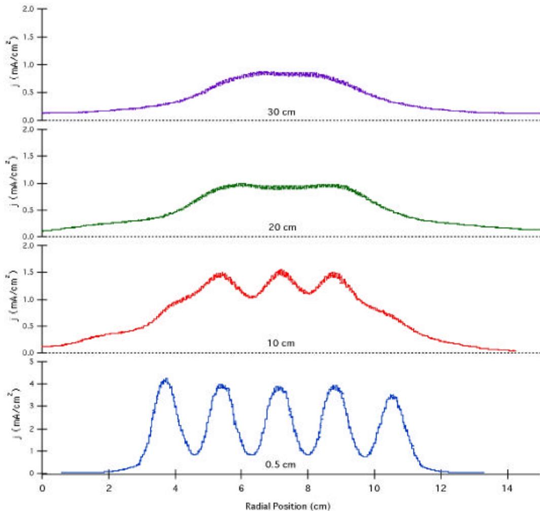
Figure 5 - Faraday probe traces as functions of distance downstream of accelerator grid (grid set 1 operated at 12,000 volts, net voltage and 70 mA beam current).
