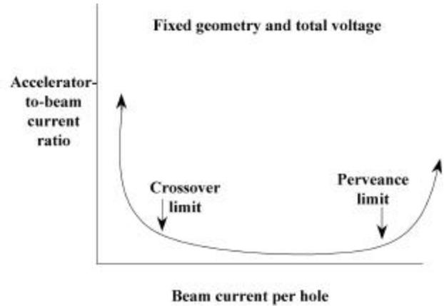
Figure 4 - Accelerator grid impingement limits.
