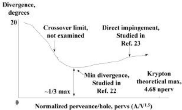
Figure 3 - Beamlet divergence as a function of normalized perveance per hole.
