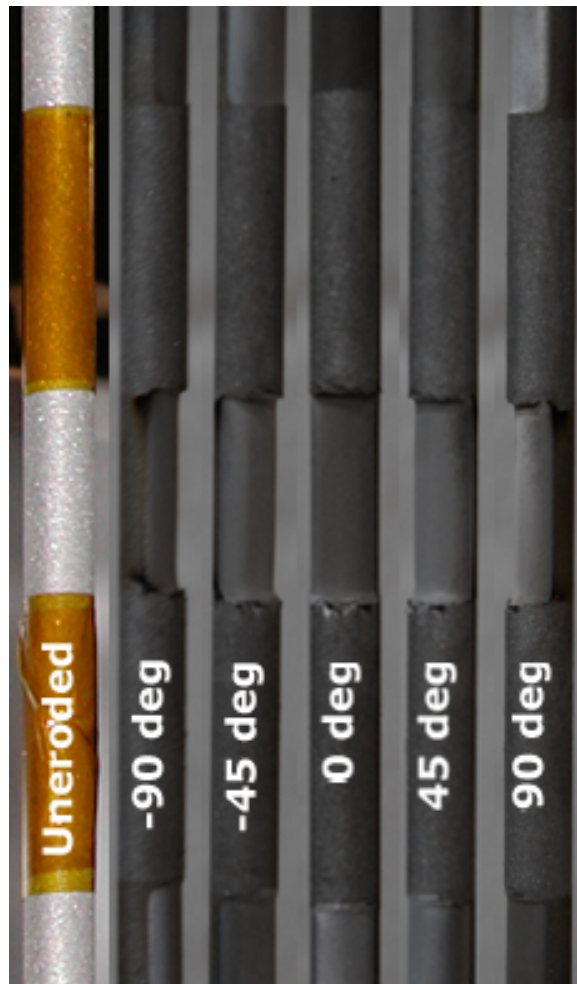
Figure 2. Aluminum rod before exposure (left) followed by 72 hour erosion photos ranging from -90 degrees to +90 degrees from incidence.
