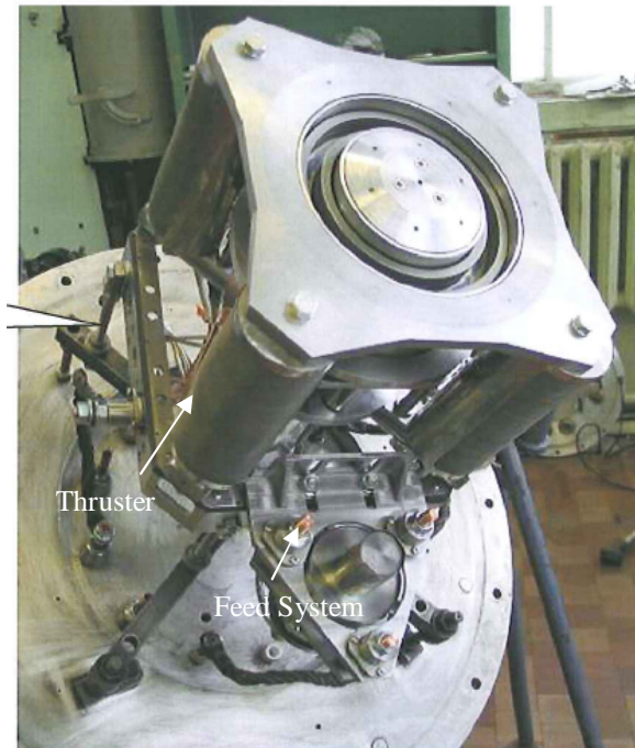
Figure 2. Fully assembly VHITAL-160 thruster attached to mounting flange in TsNIIMASH test facility 9 .
