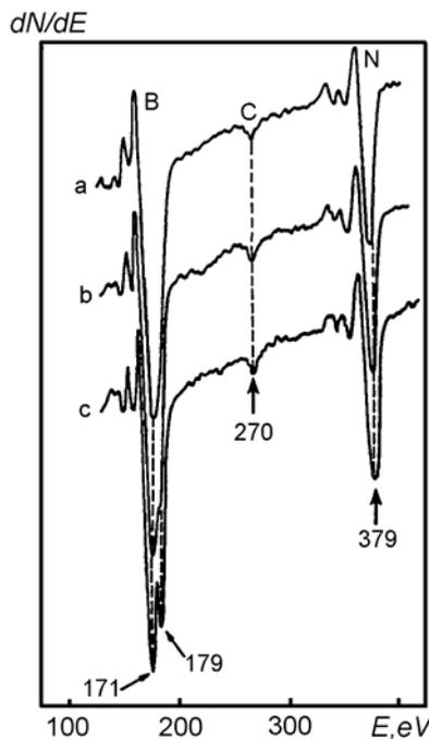
Figure 4. Auger spectra measured for the boron nitride surface at  $T = 1200 \text{ K}$  after electron irradiation with the doses  $D = 0$  (a),  $8 \cdot 10^{19}$  (b), and  $5 \cdot 10^{20} \text{ cm}^{-2}$  (c).
