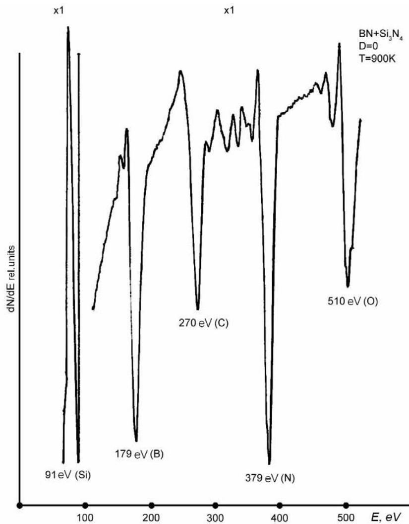
Figure 10. Energetic spectrum of Auger electrons from  $\text{BN}+\text{Si}_3\text{N}_4$  ceramic under  $T=900\text{K}$  without electron irradiation.
