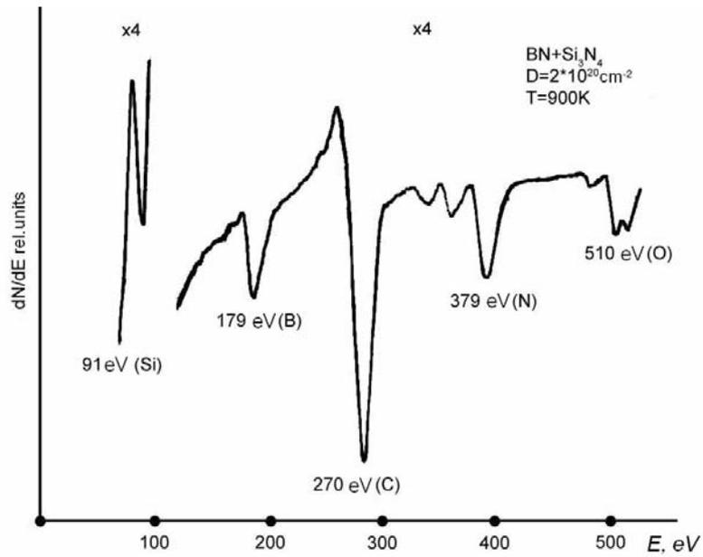
Figure 9. Energetic spectrum of Auger electrons from  $\text{BN}+\text{Si}_3\text{N}_4$  ceramic under  $T=900\text{K}$  after electron irradiation with energy  $E=3\text{ keV}$ , dose  $D=2\cdot 10^{20}\text{ cm}^{-2}$ .
