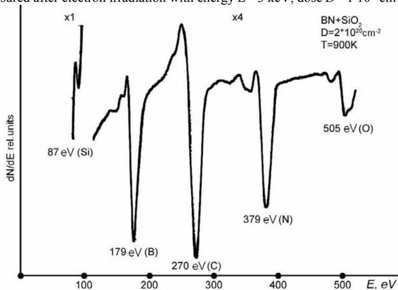
Figure 14. Energetic spectrum for Auger – electrons coming out of BN+SiO<sub>2</sub> ceramic under  $T=900\text{K}$  measured after electron irradiation with energy  $E=3\text{ keV}$ , dose  $D=2\cdot 10^{20}\text{ cm}^{-2}$ .
