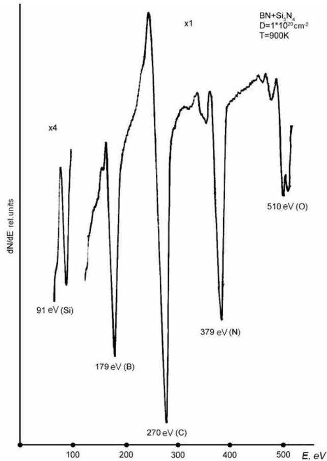
Figure 8. Energetic spectrum of Auger electrons from  $\text{BN}+\text{Si}_3\text{N}_4$  ceramic under  $T=900\text{K}$  after electron irradiation with energy  $E=3\text{ keV}$ , dose  $D=1\cdot 10^{20}\text{ cm}^{-2}$ .
