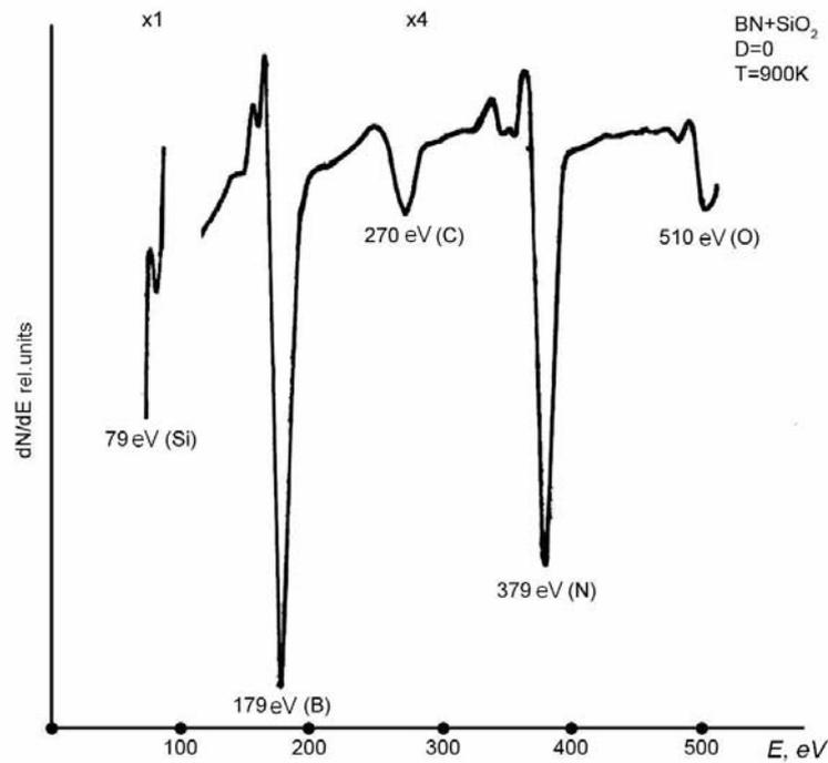
Figure 15. Energetic spectrum for Auger – electrons coming out of BN+SiO<sub>2</sub> ceramic under  $T=900\text{K}$  without electron irradiation.
