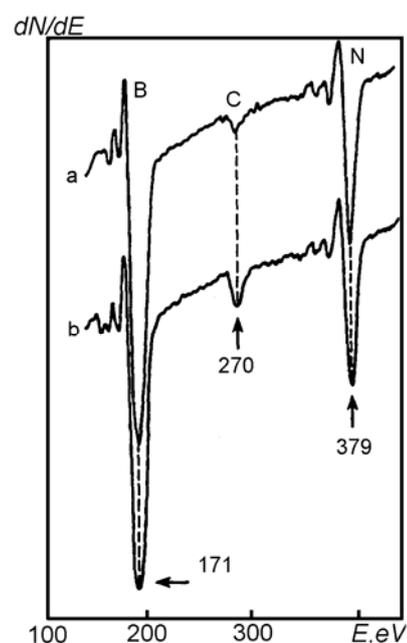
Figure 5. The same as in fig. 4 at  $T = 300 \text{ K}$  before (a) and after (b) electron irradiation with the dose of  $5 \cdot 10^{20} \text{ cm}^{-2}$ .
