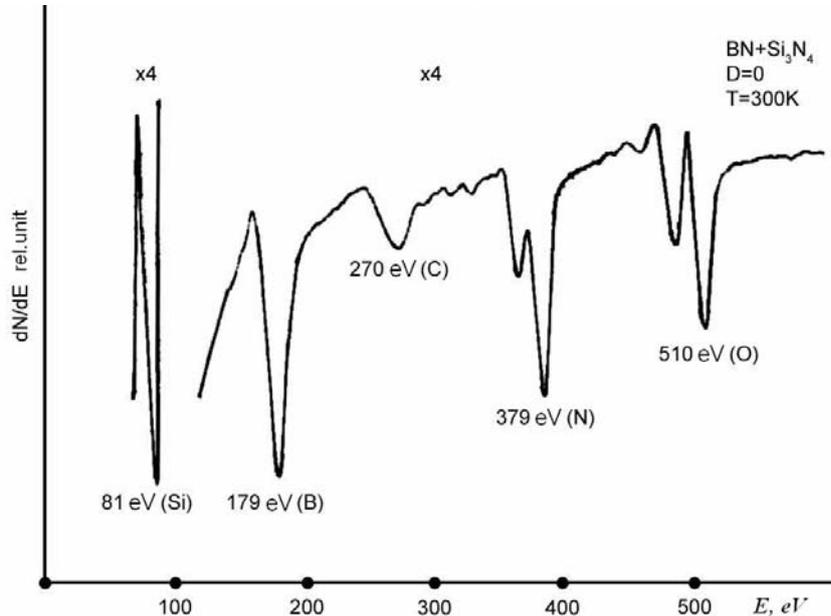
Figure 6. Energetic spectrum of Auger electrons from BN+Si<sub>3</sub>N<sub>4</sub> ceramic under  $T=300$ K measured before electron irradiation.
