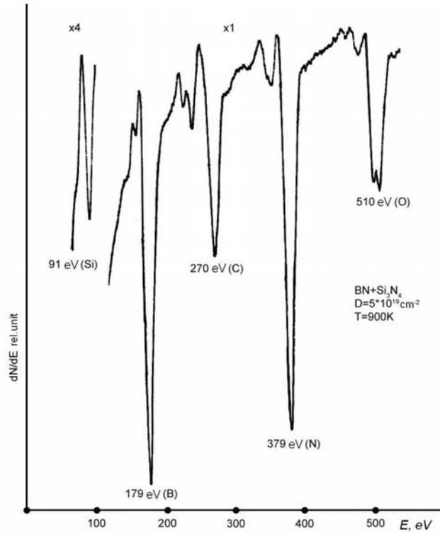
Figure 7. Energetic spectrum of Auger electrons from  $\text{BN}+\text{Si}_3\text{N}_4$  ceramic under  $T=900\text{K}$  after electron irradiation with energy  $E=3\text{ keV}$ , dose  $D=5\cdot 10^{19}\text{ cm}^{-2}$ .
