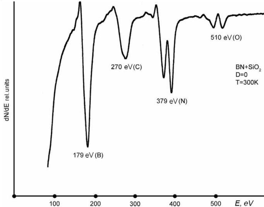
Figure 11. Energetic spectrum for Auger – electrons coming out of BN+SiO<sub>2</sub> ceramic under  $T=300\text{K}$  measured before electron irradiation.
