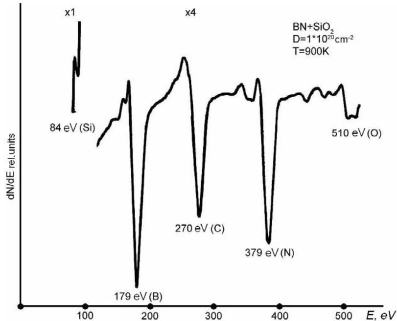
Figure 13. Energetic spectrum for Auger – electrons coming out of BN+SiO<sub>2</sub> ceramic under  $T=900\text{K}$  measured after electron irradiation with energy  $E=3\text{ keV}$ , dose  $D=1\cdot 10^{20}\text{ cm}^{-2}$ .
