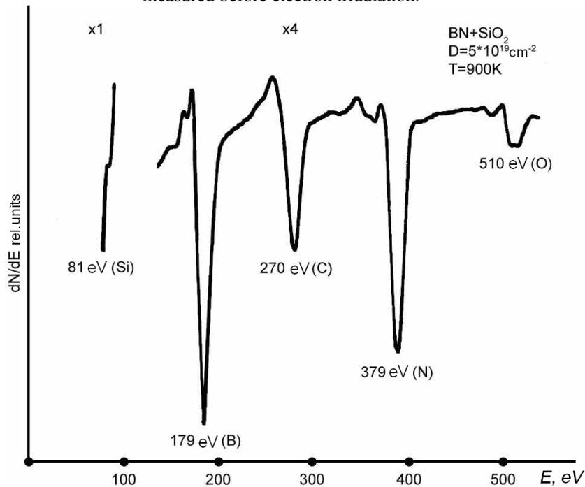
Figure 12. Energetic spectrum for Auger – electrons coming out of BN+SiO<sub>2</sub> ceramic under  $T=900\text{K}$  measured after electron irradiation with energy  $E = 3 \text{ keV}$ , dose  $D = 5 \cdot 10^{19} \text{ cm}^{-2}$ .
