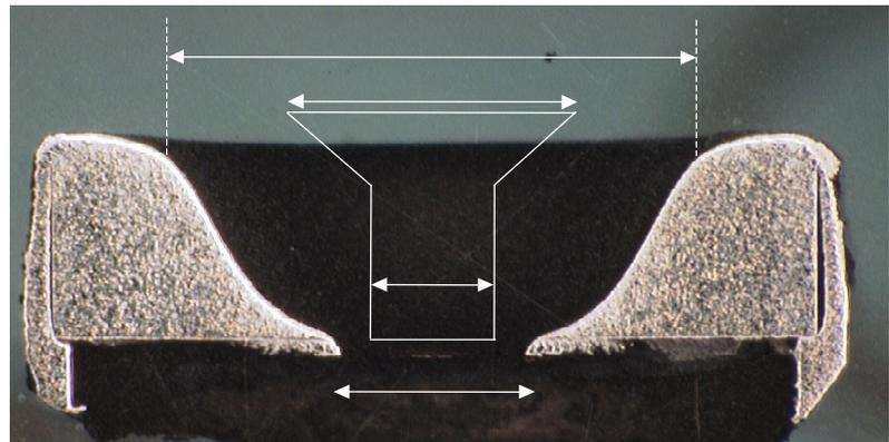
**Figure 5. Cross sectional view of the 13Q2 discharge cathode orifice plate at the end of life. The outline of the original orifice cross-section with the 45° chamfer is also shown**
