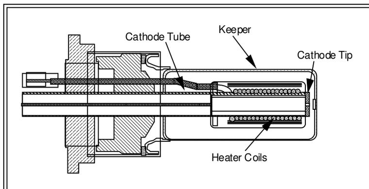
**Figure 2. Schematic of the Cathode Assembly**
