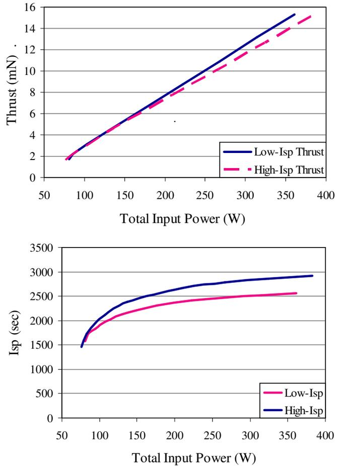
**Figure 10. Thrust and Isp versus input power for the 8-cm design.**
