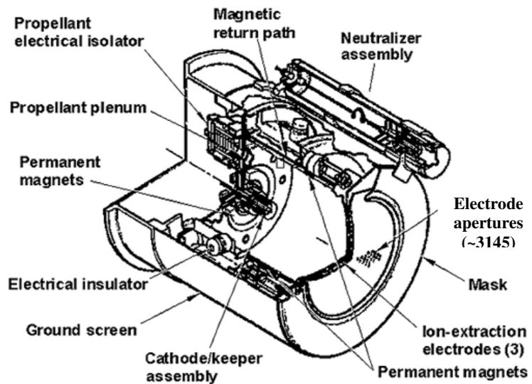
**Figure 1. XIPS thruster schematic illustration**
