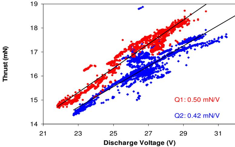
**Figure 4. Correlation of Thrust vs. Discharge Voltage**
