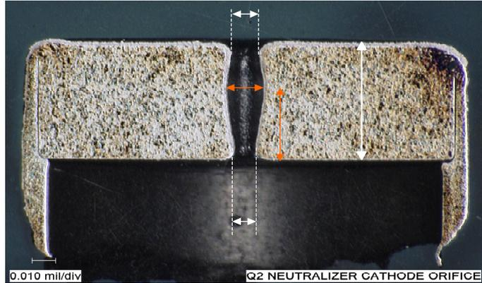
**Figure 6. Cross sectional view of the Q2's neutralizer cathode orifice plate at the end of life. The outline of the original orifice diameter is shown**
