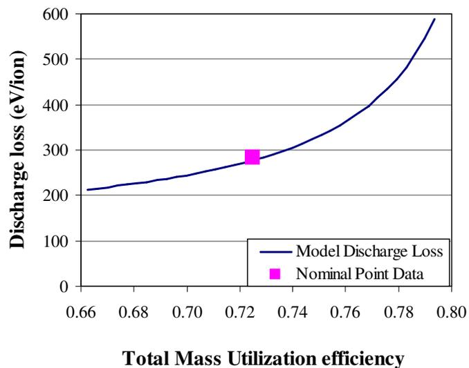
**Figure 7. Discharge loss versus mass utilization efficiency calculated for the 13-cm XIPS thruster.**
