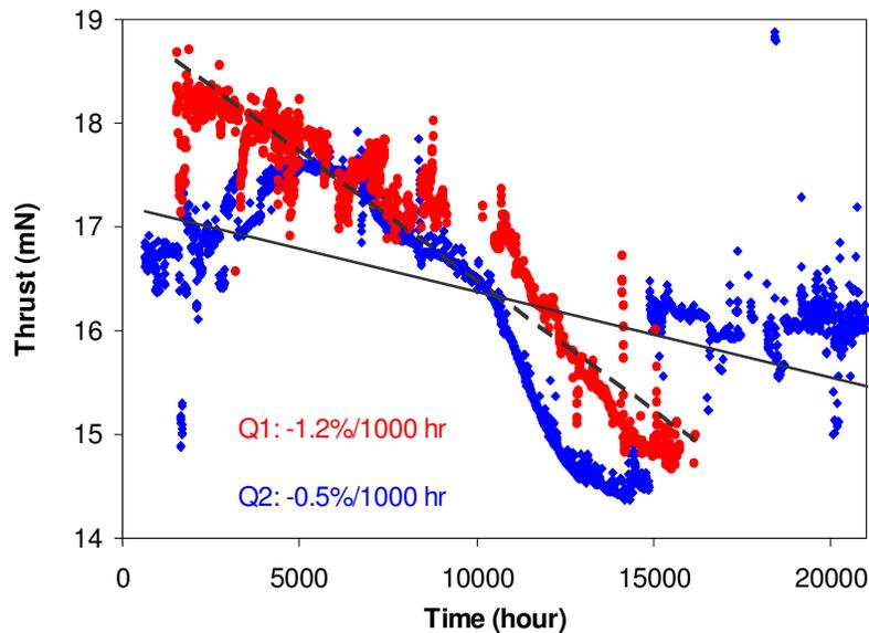
**Figure 3. Temporal profile of Thrust, averaged over each burn cycle, for Q1 and Q2 over their life tests**
