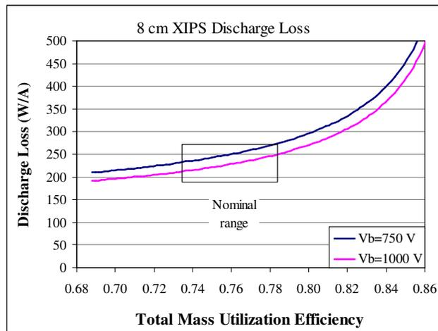
**Figure 9. Discharge loss versus mass utilization efficiency predicted for the 8-cm XIPS thruster.**
