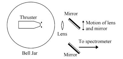
Figure 3. Plan view of the optical detection setup for Doppler spectroscopy.
