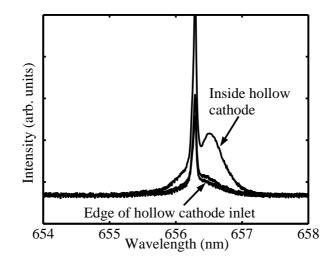
Figure 5. Doppler Spectroscopy of the inlet side of the hollow cathode showing the red Doppler shift within the centre (higher intensity) and edge (lower intensity) of the cathode. The Doppler shift outside of the inlet side (within the discharge) is also shown but almost coincides with the spectrum from the cathode edge.
