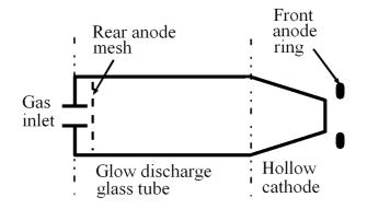
Figure 1. The Charge Exchange Thruster (CXT)
