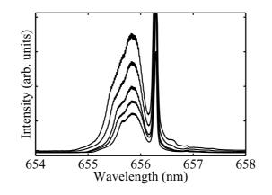
Figure 4. Doppler Spectroscopy of the Exit Nozzle of the CXT for increasing voltages (and currents) across the discharge. The voltages (and currents) from the lowest to the highest intensity Doppler shifted spectra are 4.01 kV (10 mA), 4.85 kV (15 mA), 5.01 kV (20 mA), 6.14 kV (31 mA), and 7.15 kV (45 mA), respectively.
