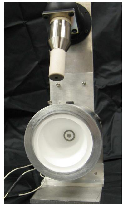
**Figure 4. Assembled DCHT and Busek hollow cathode prior to initial testing.**
