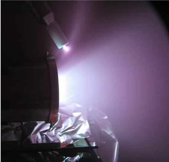
(a) Visible discharge of the first successful DCHT test.
