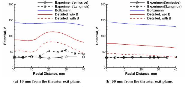
Figure 5. Radial profiles of plasma potential.
