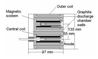
Figure 1. Schematic of the D55 anode-layer Hall thruster.
