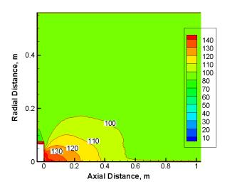
Figure 3. Contours of plasma potential (in V), the Botlzmann model
