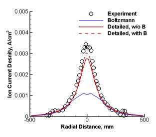
Figure 8. Radial profiles of ion current density at 500 mm from the thruster exit plane
