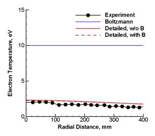
Figure 12. Radial profiles of electron temperature at an axial distance of 500 mm from the thruster
