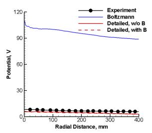
Figure 6. Radial profiles of plasma potential at 500 mm from the thruster exit plane
