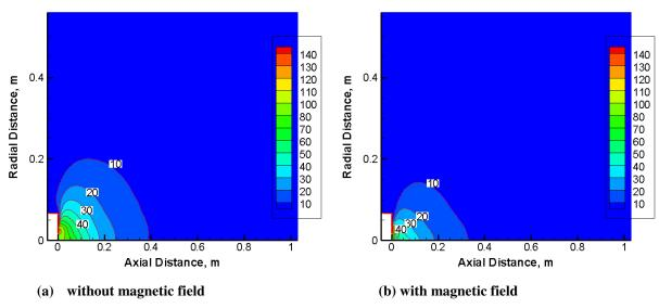
Figure 4. Contours of plasma potential (in V), the Detailed model
