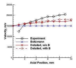
Figure 13. Axial components of ion velocity at a radial position of 27.5 mm.
