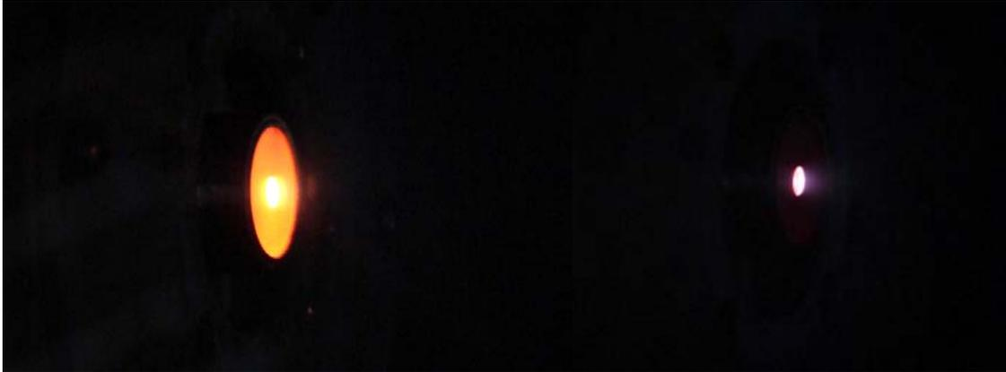
Figure 16 T5 HCT during operation with argon at 70.3W (3.2A) at 21V with 0.05mgs<sup>-1</sup> (left) and 12.8W (0.8A) at 15V with 0.8mgs<sup>-1</sup> (right)
