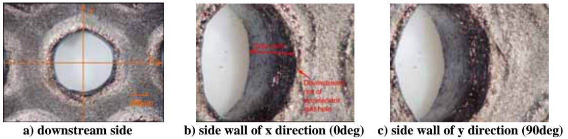
Figure 14. Close-up view of center hole of screen grid (position: r16). z axis is defined in the direction toward from space. b ) and c ) show side wall of screen grid when z axis is inclined to 45 degrees.
