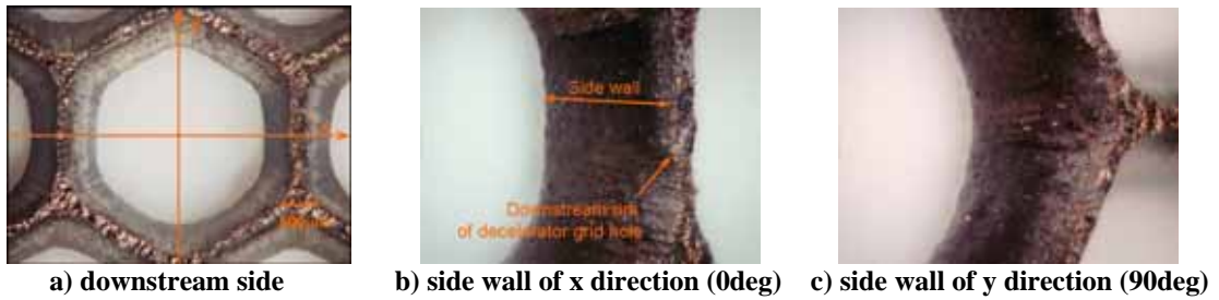
Figure 18. Close-up view of center hole of screen grid (position: r16). z axis is defined in the direction toward from space. b) and c) show side wall of screen grid when z axis is inclined to 45 degrees.
