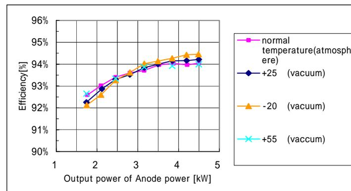
Figure 4. Power efficiency of the anode conditioner (at output voltage :350V)
