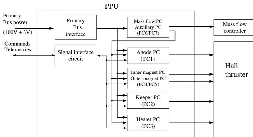
Remark: The EM1 PPU consists of PC1, PC2, PC4, PC5, and Primary Bus interface part.
