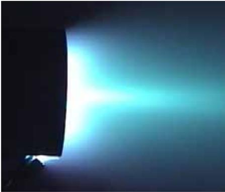
Figure 6. EM1 hall thruster 250mN-thrust operation with EM1 PPU
