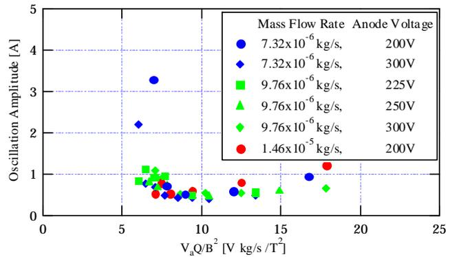
Figure 7. Behavior of a part of low frequency in discharge current characteristic
