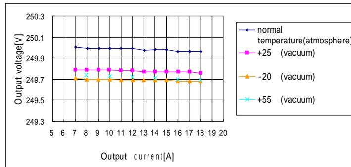
Figure 3. Load regulation of the anode conditioner
