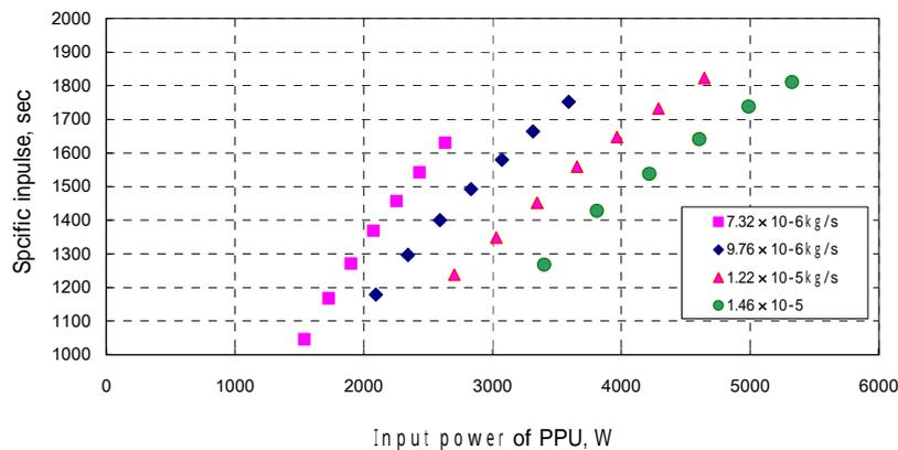
Figure 8. Specific impulse characteristics
