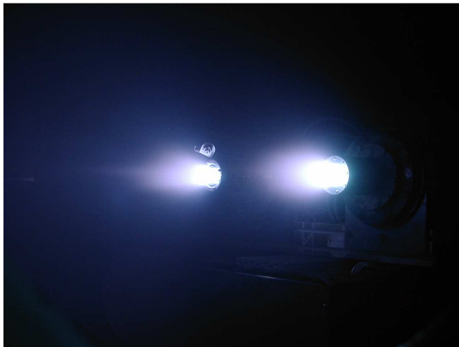
Figure 4. Two module HEMP-T cluster during test firings. The cluster is operated on one common anode line of a single PSCU. A hollow cathode neutralizer is mounted above the left thruster.
