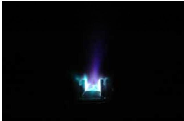
Figure 3. Operation of the test model thruster. When operated as a PP-PPT.
