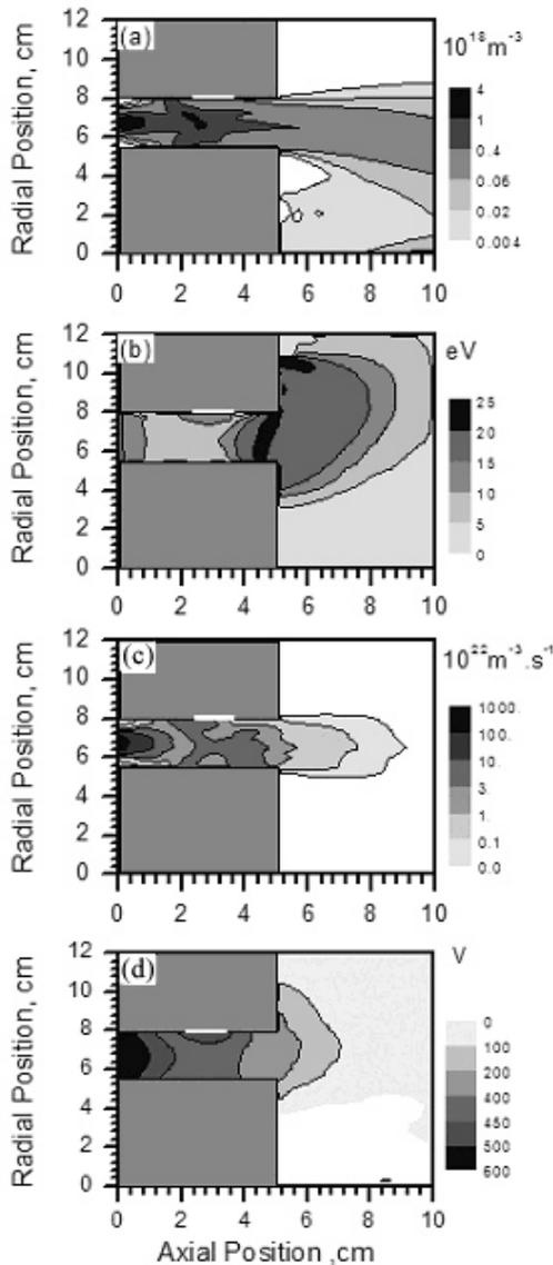
**Figure 4: 2D plasma characteristics in the case:  $V_i=100V$ ,  $V_a=500V$  and a mass flow rate of  $10 \text{ mg.s}^{-1}$ ; a) plasma density ( $\times 10^{18} \text{ m}^{-3}$ , log scale); b) electron energy (eV); c) ionization source term ( $\times 10^{22} \text{ m}^{-3}.\text{s}^{-1}$ , log scale); e) potential (V) - the white box represents the intermediate electrode.**
