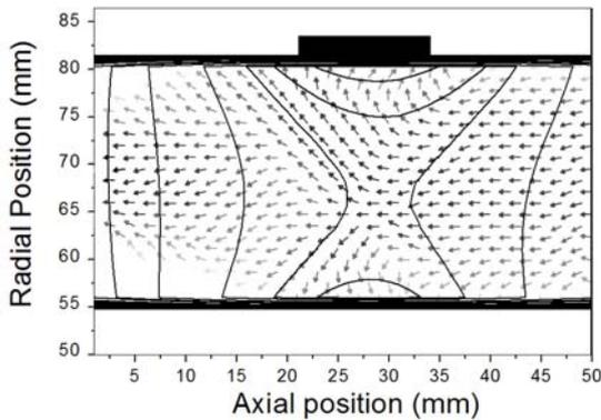
**Figure 5: Electrons flow in channel for a double stage configuration (10 mg.s<sup>-1</sup>,  $V_i=100V$  and  $V_a=500V$ ). Black lines show some magnetic field lines. The intensity of the flux is indicated by the grey level of the arrows (darker arrow corresponds to a larger flux. maximum value  $10^{22} \text{ m}^{-2} \cdot \text{s}^{-1}$ )**
