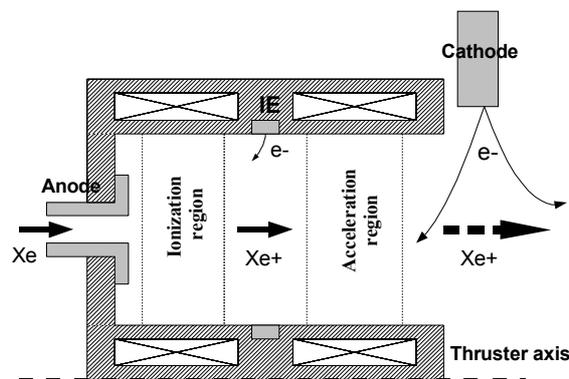
Figure 1: Schematic view of the DSHET with the Intermediate Electrode (IE) and the four coils configuration.
