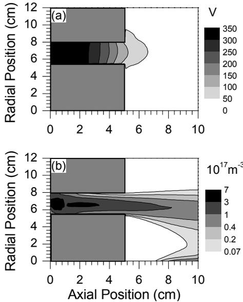
**Figure 3: a) potential (V) and b) plasma density ( $\times 10^{17} \text{ m}^{-3}$ , log scale) for a nominal single stage mode simulation: mass flow rate  $4.7 \text{ mg.s}^{-1}$  and  $V_d=350\text{V}$ .**
