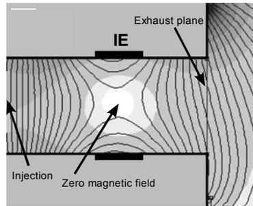
**Figure 2: Double stage 2D magnetic field configuration and lines – the zero magnetic field is visible in the middle of the channel.**
