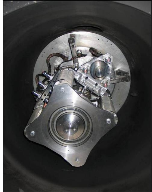
Figure 25. The thruster placed in vacuum tank.
