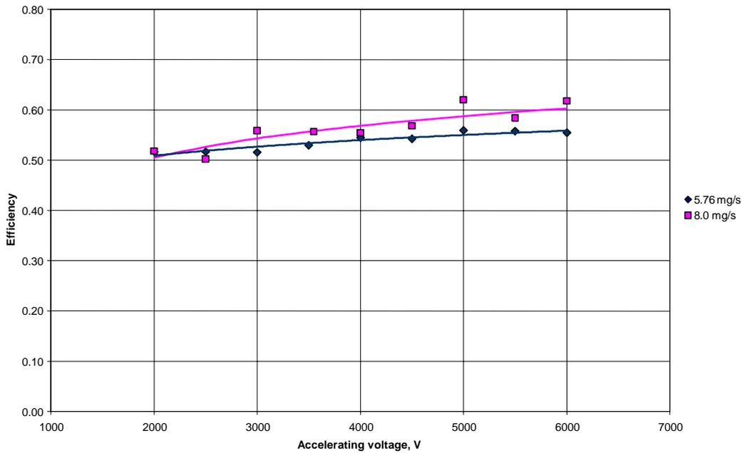
Figure 32. Dependence of the efficiency on accelerating voltage at 5.76 and 8.0 mg/sec of bismuth flow rate.
