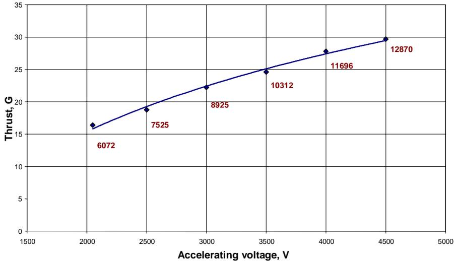
**Figure 29. Dependence of the thrust on accelerating voltage.**
