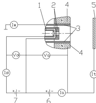
Figure 2. Two-stage thruster scheme.
