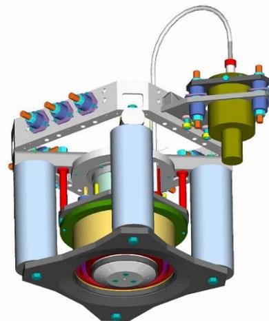
**Figure 18. Feed system fastening in case of vertical thruster orientation.**
