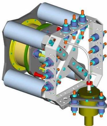
**Figure 17. Feed system mounting in case of horizontal thruster orientation.**
