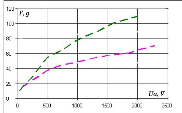
**Figure13. Thrust vs Accelerating Voltage .**
