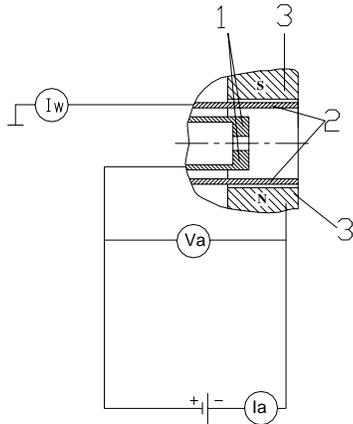
Figure 1. One-stage thruster scheme.
