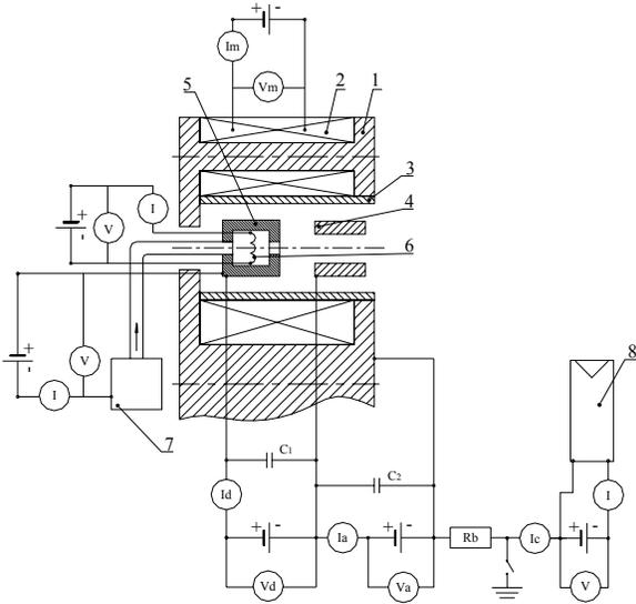
**Figure 20. The electrical schematic for the bismuth thruster with the cathode-neutralizer.**
