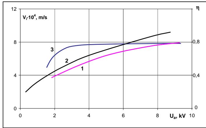
**Figure 6. Ion Velocity & Thruster Efficiency vs Accelerating Voltage.**
