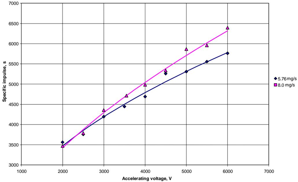
Figure 31. Dependence of specific impulse on accelerating voltage at 5.76 and 8.0 mg/sec of bismuth flow rate.
