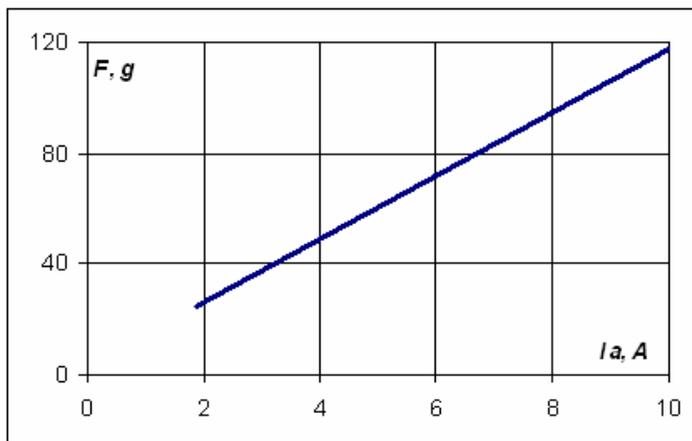
**Figure 7. Thrust vs Accelerating Current.**
