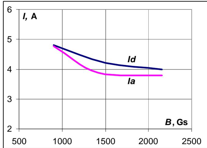
Figure 10. Discharge and accelerating current versus magnetic induction .
