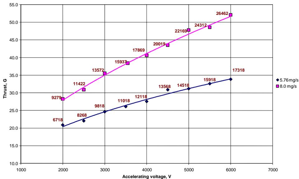
**Figure 30. Dependence of the thrust on accelerating voltage at 5.76 and 8.0 mg/sec of bismuth flow rate.**
