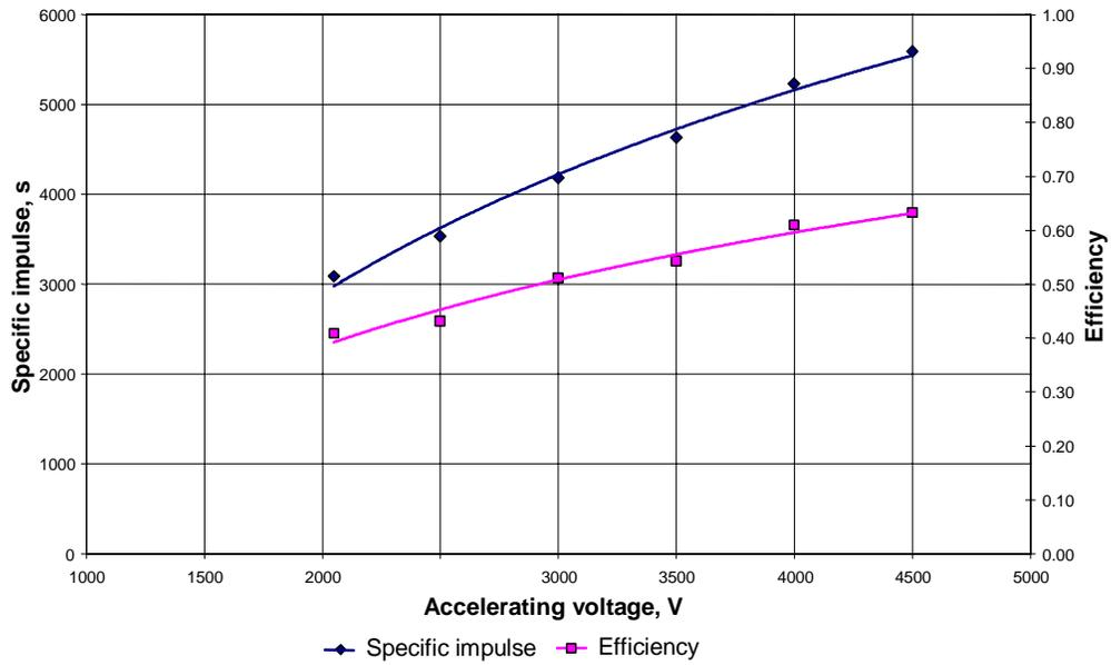
Figure 28. Dependence of specific impulse and efficiency on accelerating voltage.
