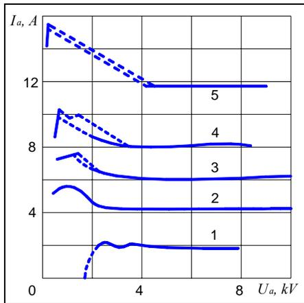
**Figure 5. Volt-Ampere Characteristics of Bismuth TAL.**
