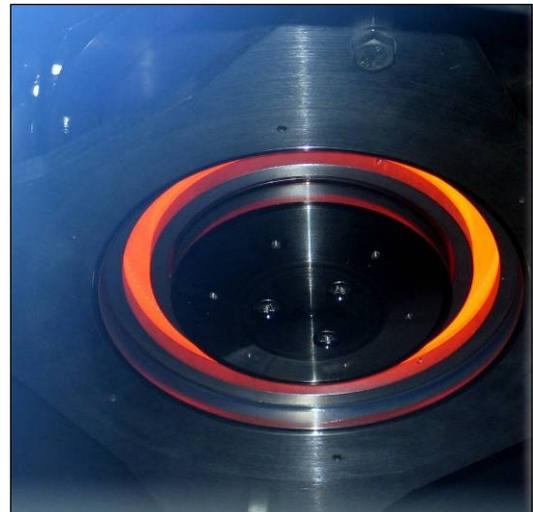
Figure 26. Thruster preheating.
