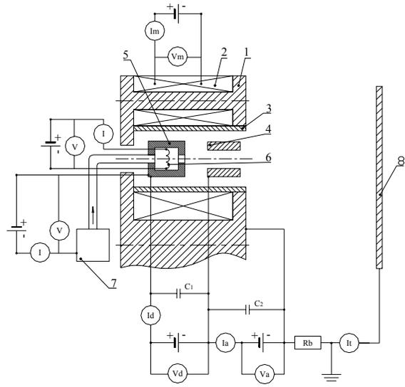
**Figure 21. The electrical schematic for the bismuth thruster with the beam target without cathode-neutralizer.**
