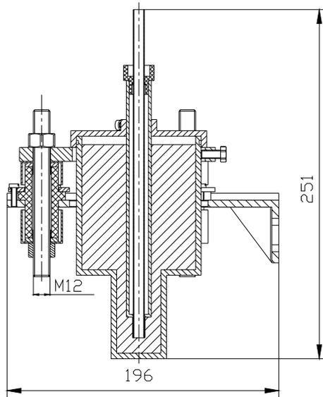
**Figure 15. Feed system basic scheme.**
