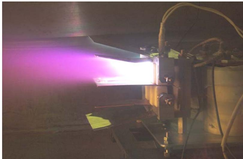
**Figure 4. Tests of the APPT laboratory model**
