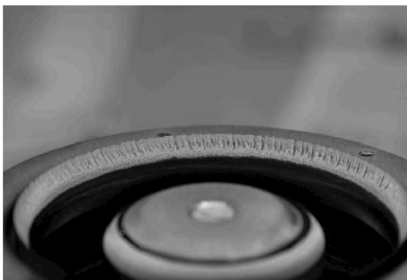
Figure 15. 1 st HET laboratory model after 500 hours of operation Insulators material - BGP
