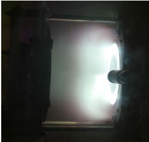
Figure 2. Operation of sputtering yield measurement apparatus.
