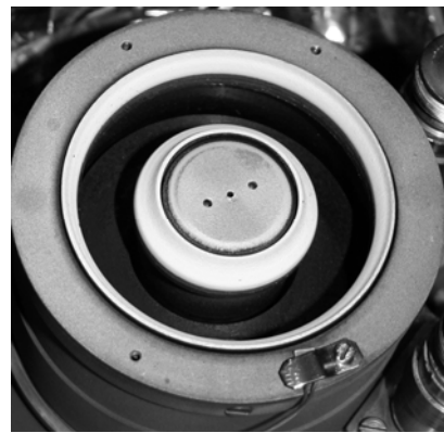
Figure 16. 3 rd HET laboratory model after 500 hours of operation Insulators material - BN-05
