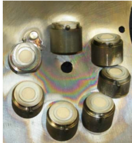
Figure 3. Mounting plate with samples and Faraday cup after exposition in plasma plume.
