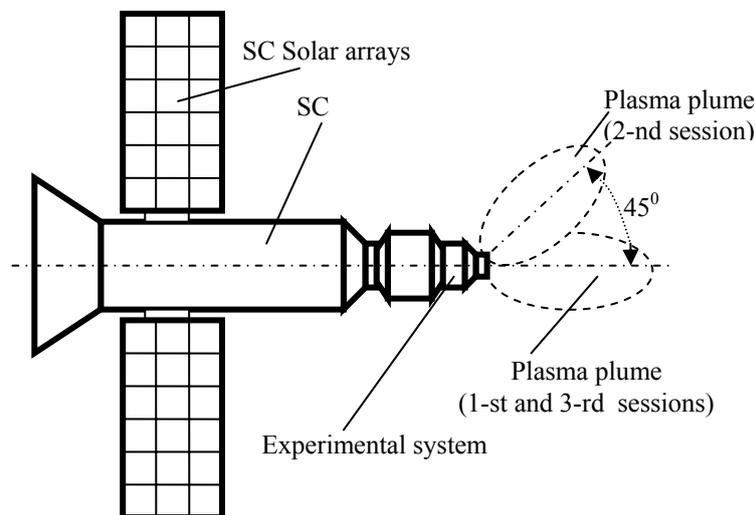
**Figure 6. “Progress M-4 “ experiment schematics**
