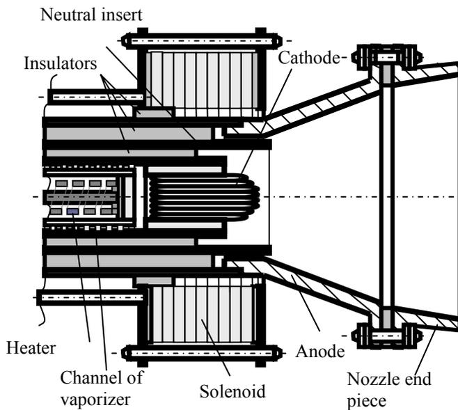
**Figure 4. Medium-power Hybrid MPDT schematics**
