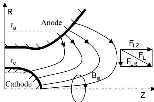
**Figure 1. Self-field MPD principle of operation**
