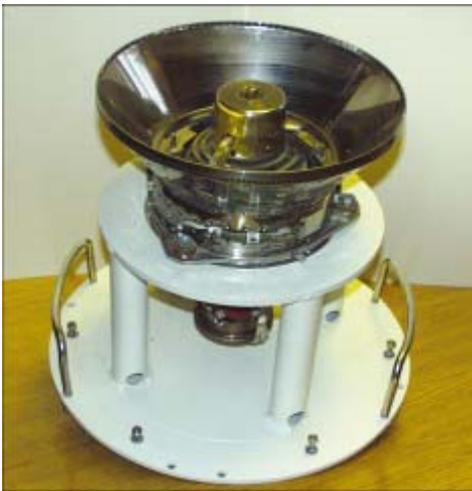
**Figure 15. A flight model of "Micron" Lithium thruster**
