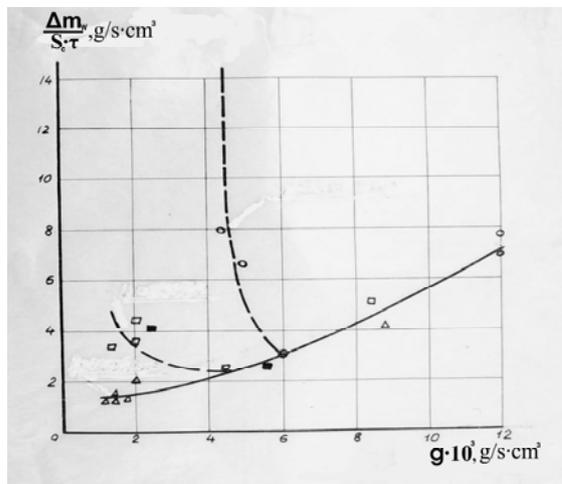
**Figure 7. The dependence of specific ablation speed of tungsten from anode on lithium mass flow rate to cathode surface ratio:  $\Delta$  - current density 100 A/cm<sup>2</sup>,  $\square$  - current density 160 A/cm<sup>2</sup> at 500 A current,  $\circ$  - current density 160 A/cm<sup>2</sup> at 5000 A current,  $\blacksquare$  - 240A/cm<sup>2</sup> at 5000 A current.**
