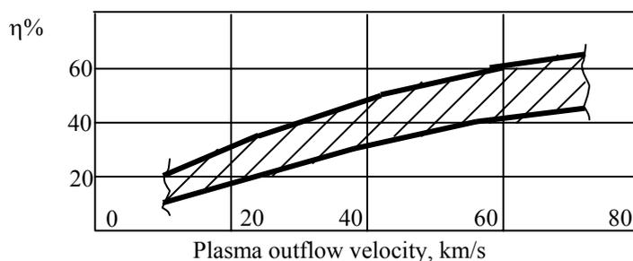
**Figure 2. Lithium MPDT efficiency as a function of outflow velocity**
