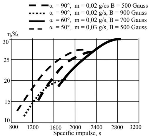
**Figure 5. Relationship between the efficiency and specific impulse at different magnetic fields and anode expansion angles**
