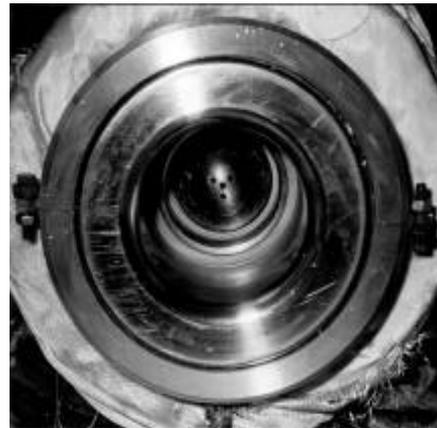
**Figure 12. Coaxial high-current MPD thruster. Figure 13. SF-MPD thruster. Picture taken in 1964**
