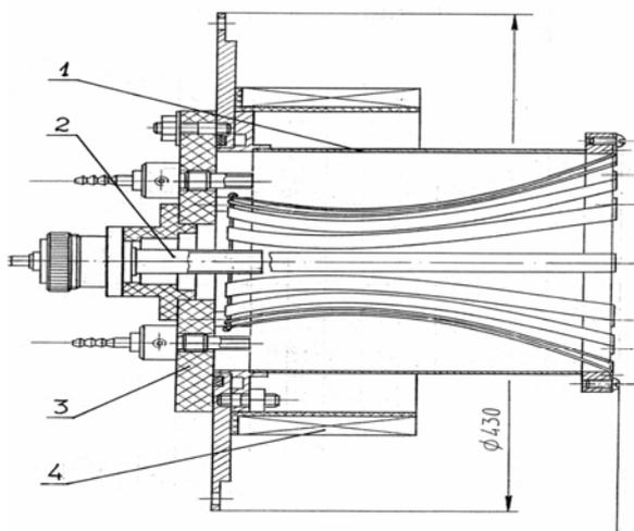
**Figure 16. Quasi-stationary MPDT for working on gaseous propellant**
