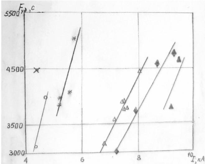
**Figure 9. MPDT specific impulse as a function of discharge current at Lithium mass flow rates: 1 – 0.026 g/s; 2 – 0.08 g/s; 3 – 0.10 g/s; 4 – 0.13 g/s; 5 – 0.24 -0.26 g/s; 6 – 0.28-0.30 g/s; 7 – 0.33-0.36 g/s**
