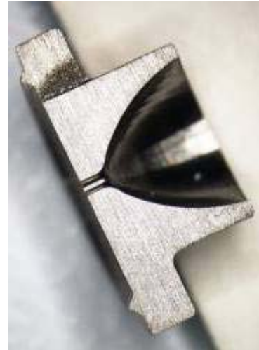
Fig. 10: LP RVN Nozzle (cutaway) close up
