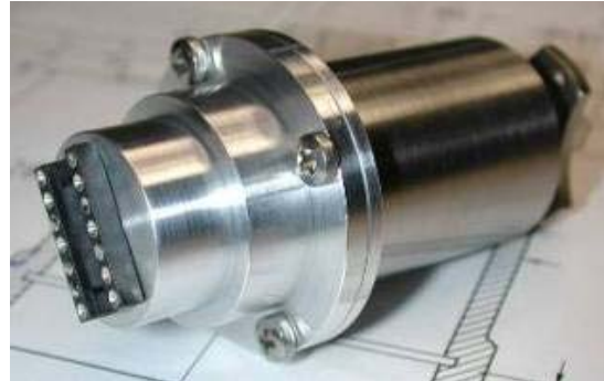
Fig. 14: Prototype of the LP RVN new design implementing the parasitic noise compensation solution
