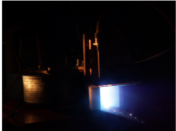
Figure 3. SIMP-LEX during one pulse for flared, tongue shaped electrode configuration.
