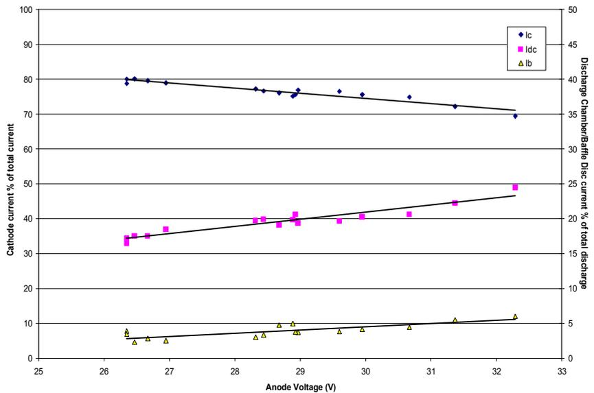
**Figure 7. T6 hollow cathode emission current fraction as a function of discharge (anode) voltage.**
