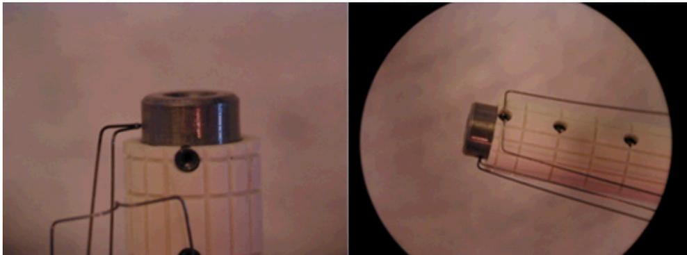
**Figure 12. Thermocouples being installed into cathode structure**
