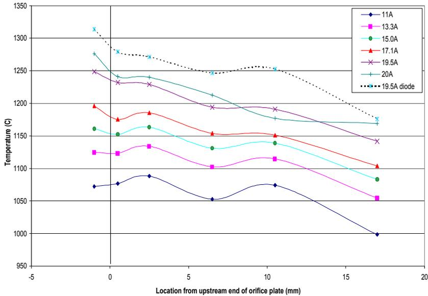
**Figure 18 T6 hollow cathode temperature profile at several engine throttle points, included for comparison is results for the diode configuration test at 19.5A.**
