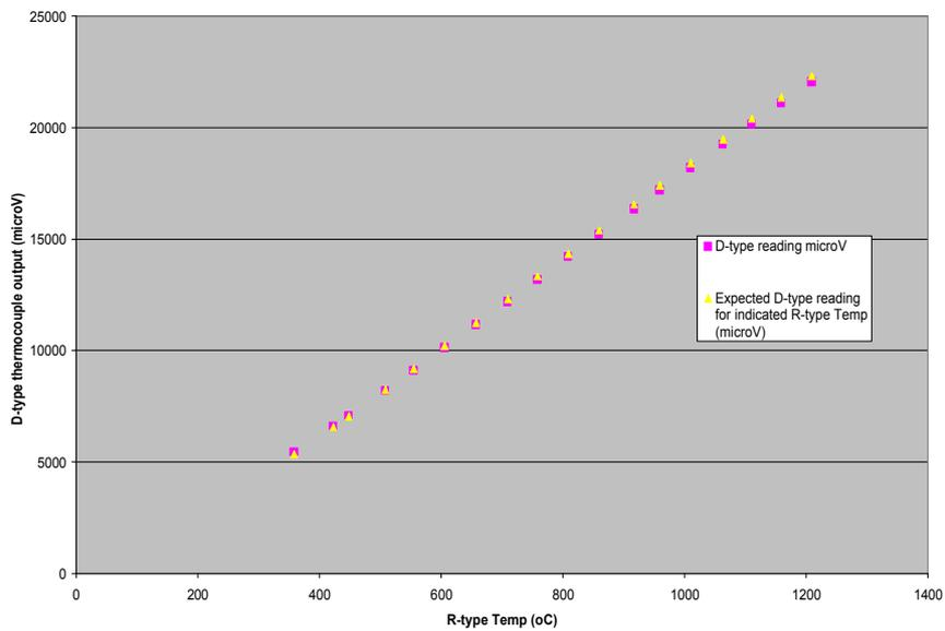
**Figure 8. Calibration curve for D-type thermocouple**
