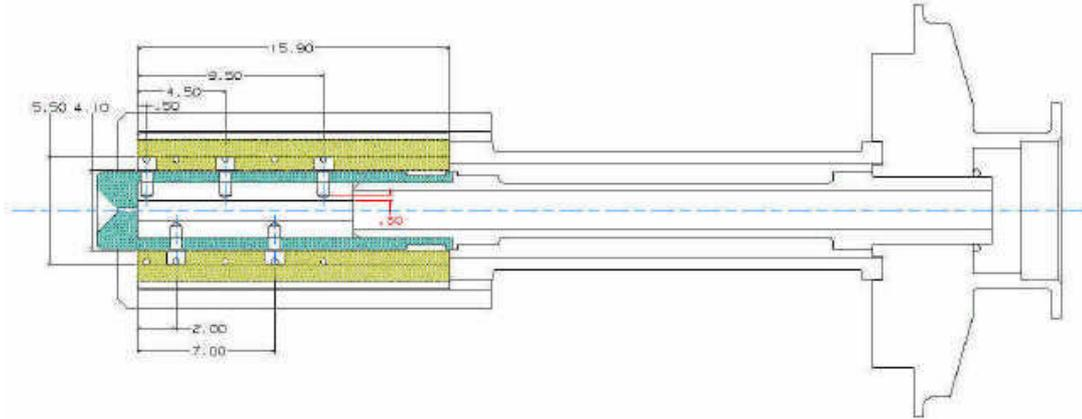
**Figure 11. Cross-section of T5 cathode showing thermocouple locations in dispenser, one thermocouple inserted into the cathode tip and five into the dispenser at 0.5, 2, 4.5, 7 and 9.5mm**
