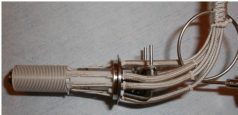
**Figure 14.** Completed instrumented T6 thermocouple with 6 D-type thermocouples
