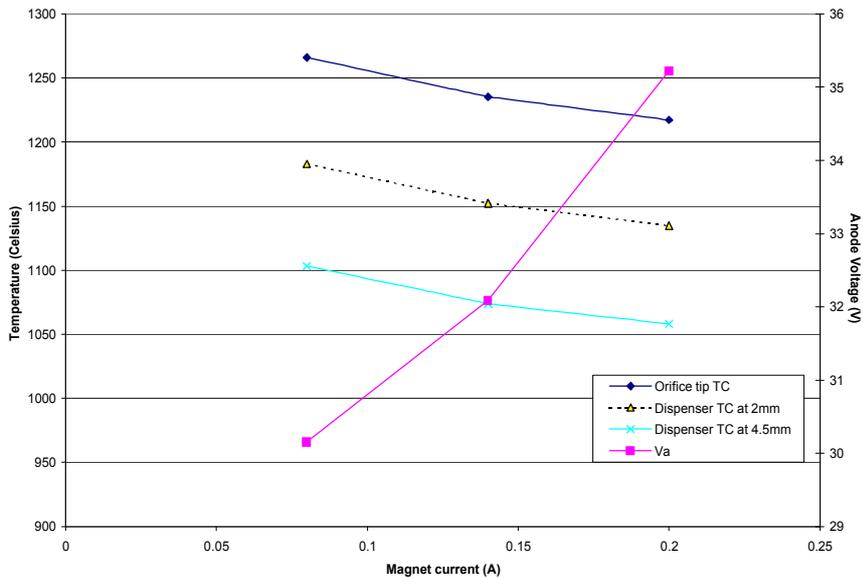
**Figure 16. Influence of magnetic field strength on measured T5 thermocouple measurements**
