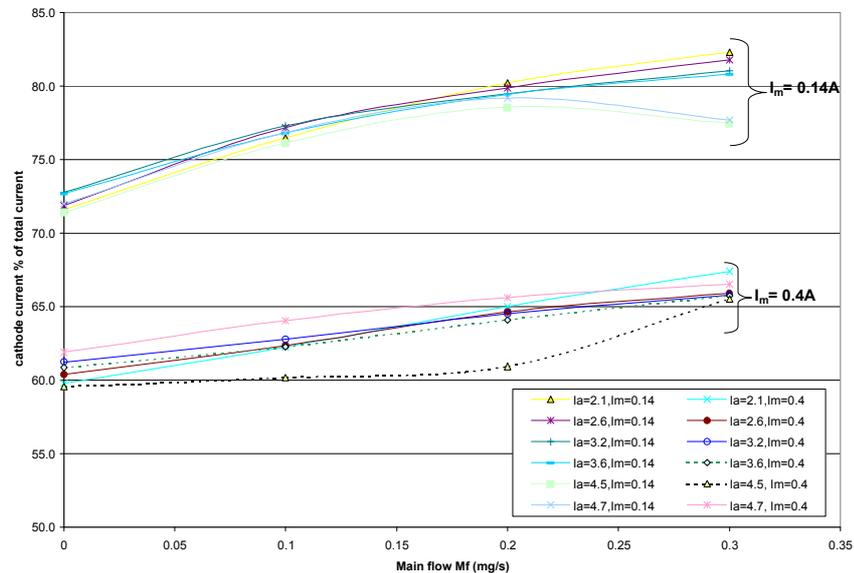
**Figure 3. T5 Cathode emission current percentage of total current as a function of main flow rate for various values of discharge and magnet currents**
