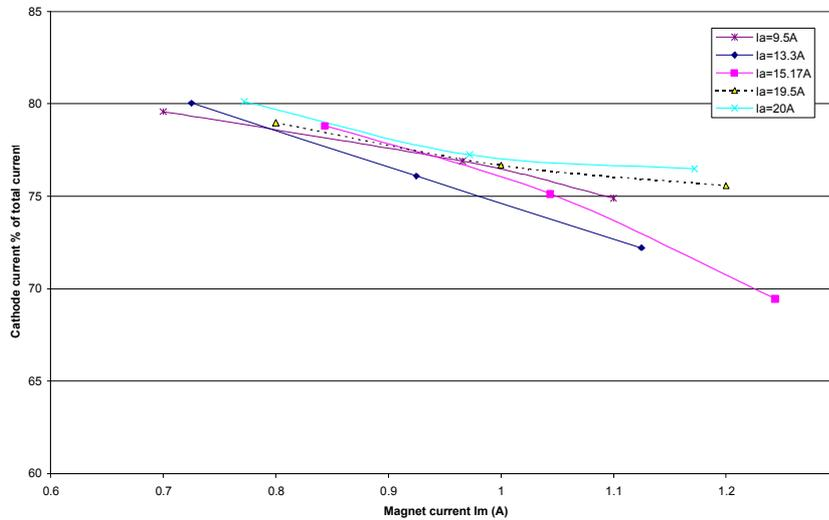
**Figure 5. Effect of magnet current on the T6 hollow cathode emission current fraction at various throttle points.**
