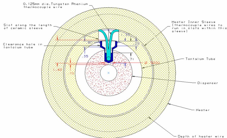
**Figure 9. Cross-section of an instrumented cathode showing cathode construction with thermocouple inserted**
