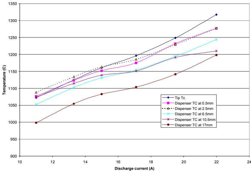
**Figure 19. T6 dispenser temperature dependence on discharge current plotted for various points along the dispenser length**
