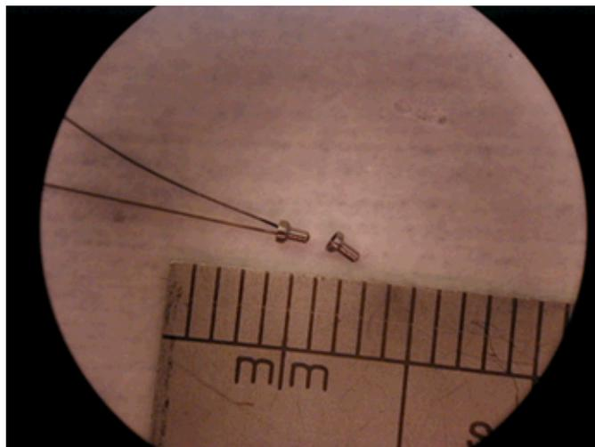
**Figure 10. Type-D thermocouple inserted in Ta sheath prior to insertion in dispenser.**
