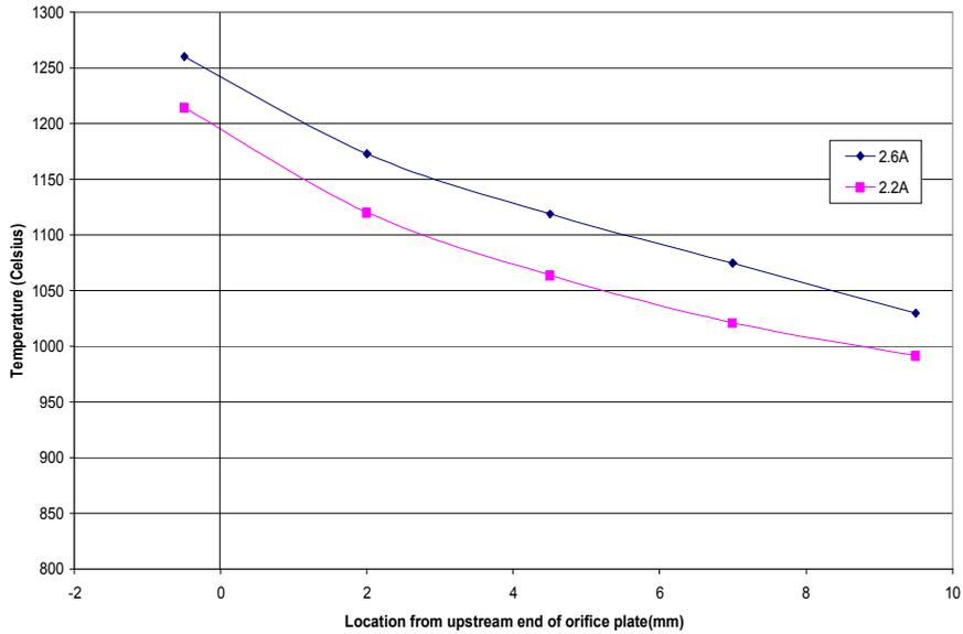
**Figure 15. T5 hollow cathode temperature profile at two discharge current settings**
