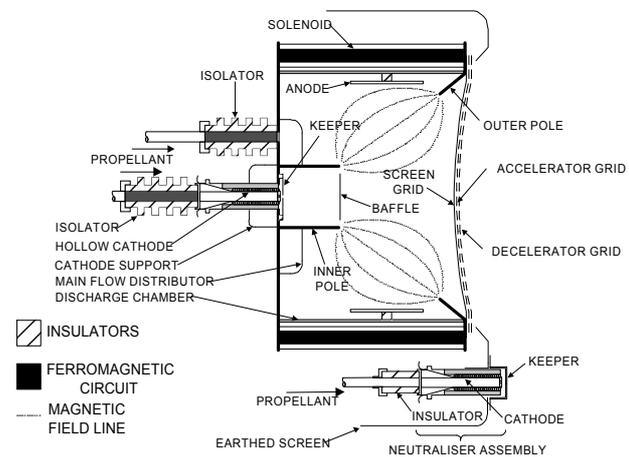
**Figure 1. A modern Kaufman-type ion thruster.**
