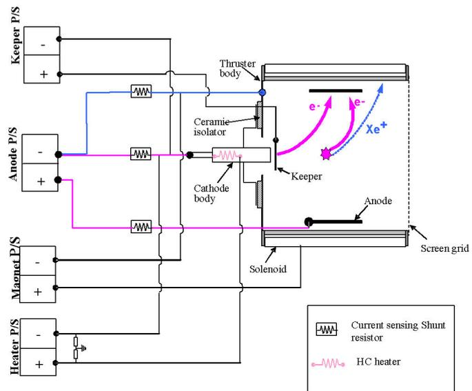
**Figure 2. A hollow cathode mounted in a full Kaufman-type thruster geometry, figure shows arrangement used to measure cathode emission current percentage of total current.**
