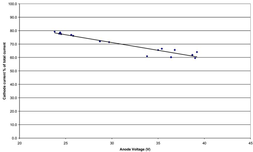
**Figure 6. T5 hollow cathode emission current fraction as a function of discharge (anode) voltage.**
