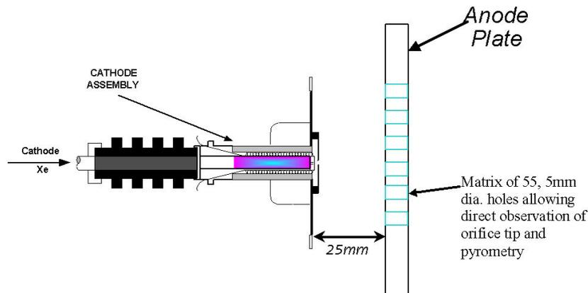
**Figure 17. Schematic of the instrumented T6 cathode in diode configuration**
