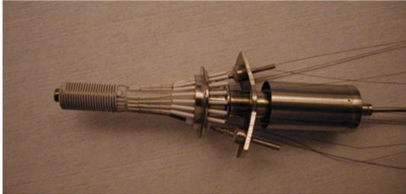
**Figure 13.** Completed instrumented T5 thermocouple with 6 D-type thermocouples
