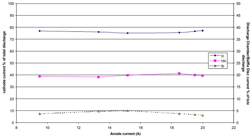
**Figure 4. T6 cathode emission current percentage of total current at various engine throttle points, also shown is the relative current balance between the baffle disc and the discharge chamber.**
