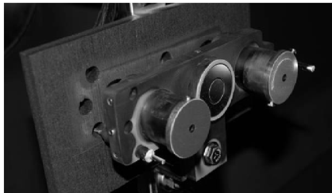
Figure 2. Plasma diagnostic array at AFRL. Probes from left to right include: Langmuir probe, RPA, nude Faraday probe, and gridded Faraday probe.
