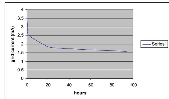
**Figure 8. Grid current as a function of time for a thrust level of 15mN and vectoring of  $7.5^\circ$**
