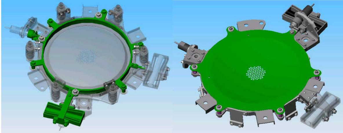
**Figure 2. T5 thruster sub assembly with actuators**
