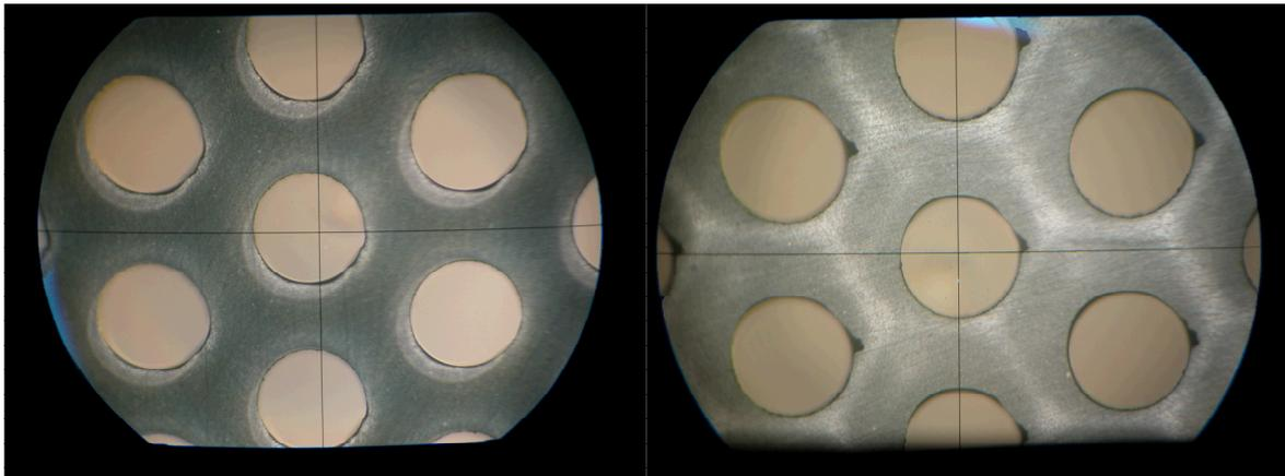
**Figure 5. Downstream and upstream faces of accel grid**
