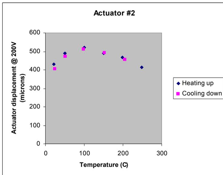
Figure 10. Actuator performance as a function of temperature
