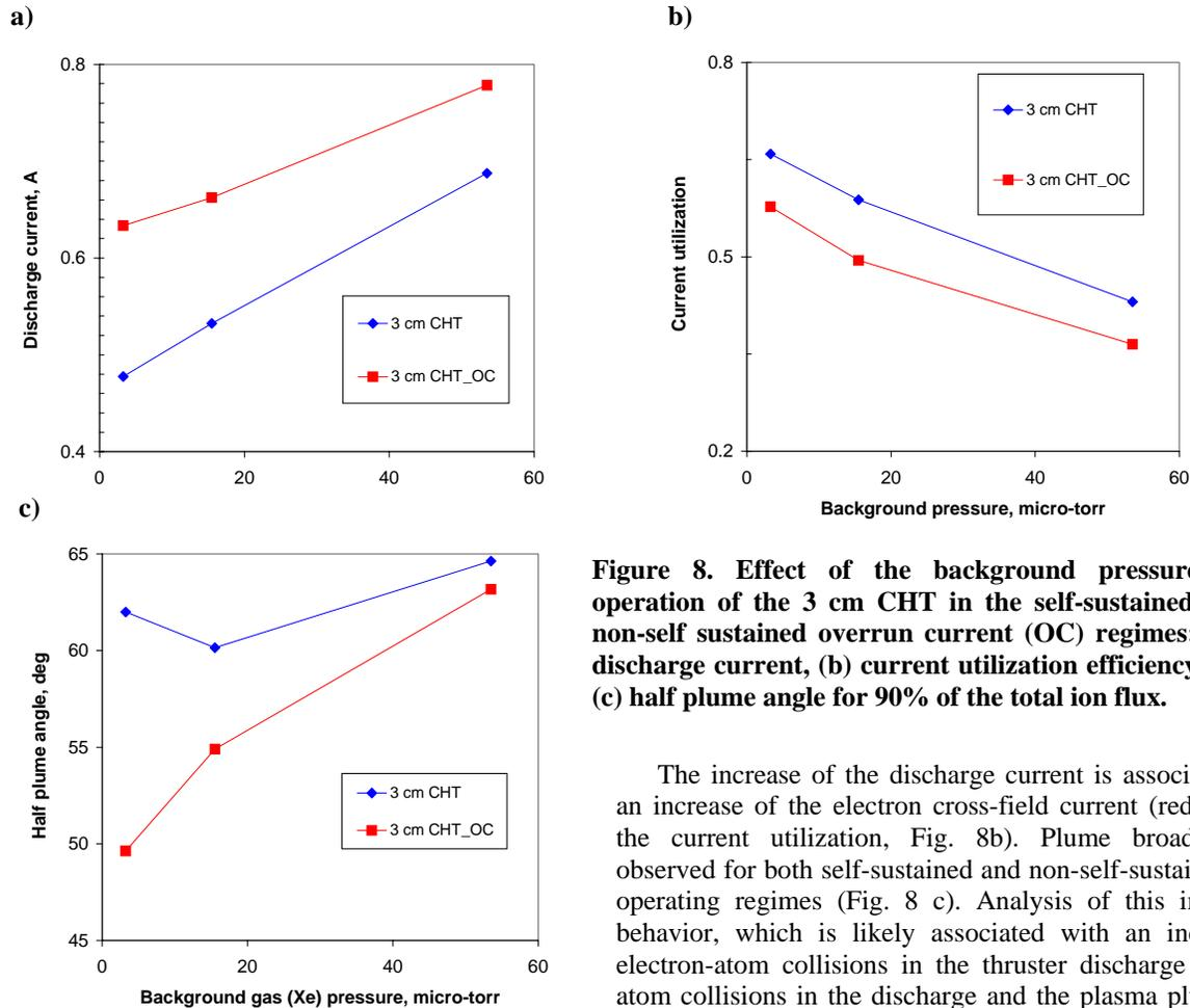
**Figure 8. Effect of the background pressure on operation of the 3 cm CHT in the self-sustained and non-self sustained overrun current (OC) regimes: (a) discharge current, (b) current utilization efficiency and (c) half plume angle for 90% of the total ion flux.**
