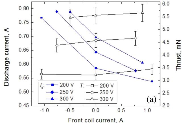
**Figure 4. The dependencies of the discharge current and thrust on the front coil current for the 2.6 cm CHT operated in background Xenon pressure less than 6 microrr.<sup>16,22</sup> Anode and cathode Xenon flow rates are 4 sccm and 2 sccm, respectively;  $I_{back} = +3A$ .  $I_{front} > 0$  ( $I_{front} < 0$ ) corresponds to the direct (cusp) magnetic field configuration.**
