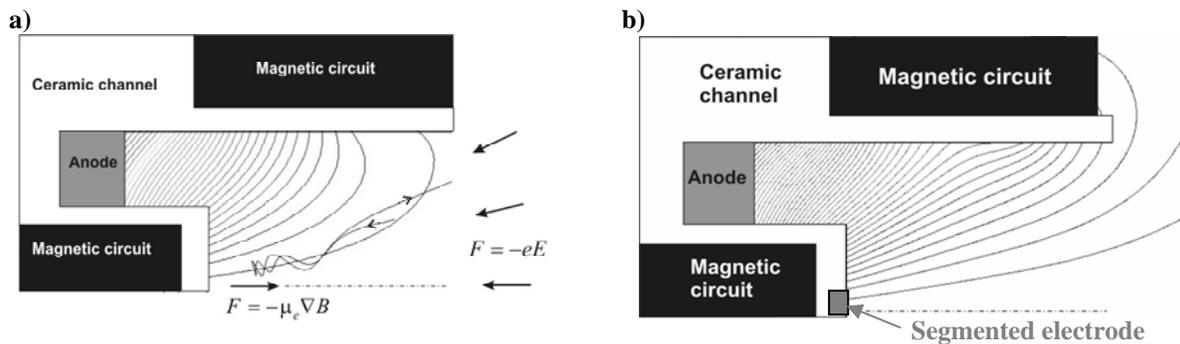
**Figure 3. Magnetic field simulations of the 100 W CHT. An illustrative electron trajectory in the cylindrical part of the channel is indicated, and the hybrid mechanism of electron trapping is schematically shown.<sup>16,28</sup> The magnetic field distribution is shown for the cusp (a) and direct (b) configurations. A segmented electrode at the axis can be used to initiate and stabilize the discharge.**
