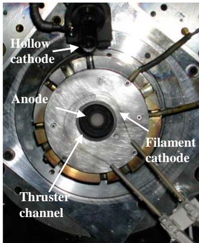
**Figure 2. The 2.6 cm, 100 W cylindrical Hall thruster. The thruster can be operated with a commercial hollow cathode or with a propellantless filament cathode. The filament is made from a tungsten wire.**
