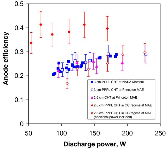
**Figure 6. The thruster (anode) efficiency for the 3 cm and 2.6 cm CHTs measured in the direct magnetic field configuration. The thrust measurements were conducted at the MAE of Princeton University<sup>5,22</sup> and at the NASA Marshall SFC.<sup>21</sup> Results for the overrun current (OC) regime<sup>23</sup> of the CHT are also shown.**
