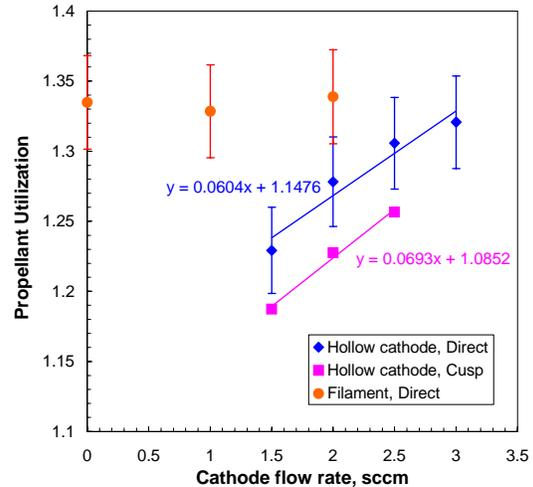
**Figure 5. Anode propellant utilization (Xenon) for the 2.6 cm CHT thruster operated with a hollow cathode and propellantless tungsten filament cathode, for direct and cusp magnetic field configurations. A linear fitting is applied to the experimental data. Background pressure did not exceed 3 micro-torr.**
