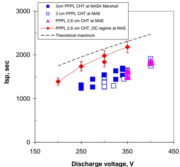
**Figure 7. Anode Isp for the 3 cm and 2.6 cm CHTs measured in the direct magnetic field configuration. Theoretical maximum,  $I_{sp}^{th} = (2e \cdot V_d / M_{ion})^{0.5} \cdot 1/g$ , is for a mono-energetic beam of single-charged ions, where  $e$  is electron charge,  $V_d$  is the discharge voltage,  $M_{ion}$  is the Xenon ion mass,  $g$  is the gravity. Results for the overrun current (OC) regime are also shown.**
