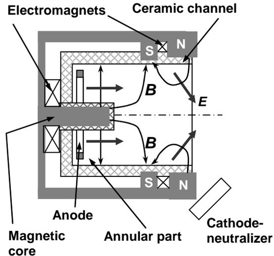
**Figure 1. Schematic of a cylindrical Hall thruster**
