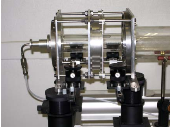
Figure 28. High power electrodeless plasma thruster prototype. The propellant injection system appears on the right. Microwave applicators have been removed. The glass tube on the right is a small vacuum vessel.
