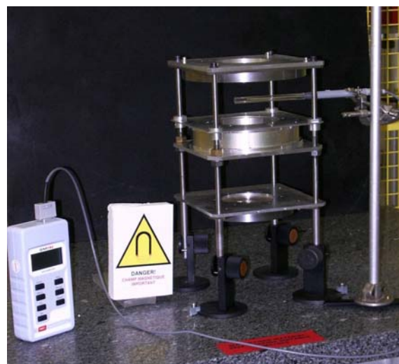
Figure 27. Magnetic field structure on magnetic field measurement bench. The structure axis is set vertically. The Hall Effect probe can be seen in the acceleration stage area.
