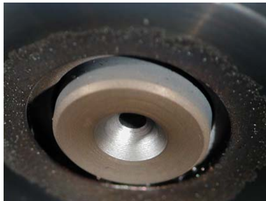
Figure 16. Photo showing condition of T6 cathode orifice post 4000 hour test
