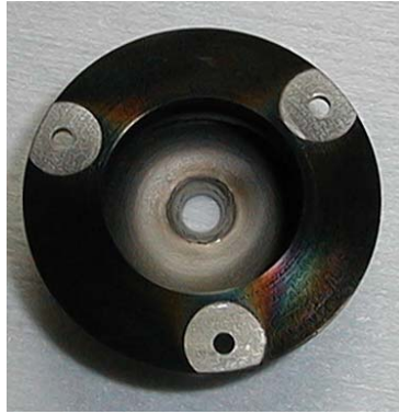
Figure 9: Photo showing condition of T5 Artemis moly keeper plate post 15,000 hour test
