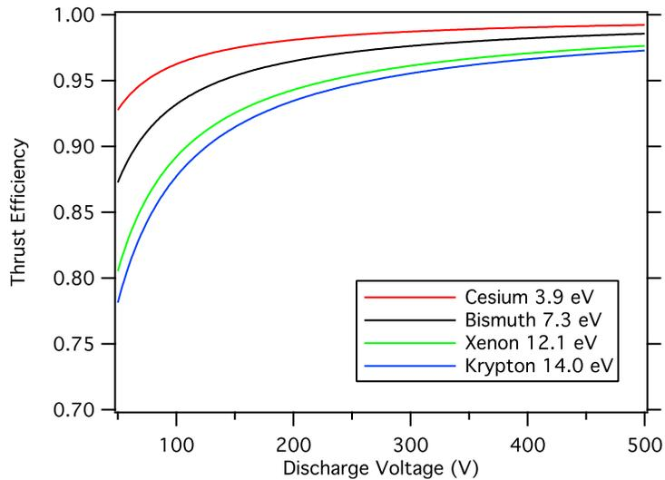
**Figure 9.** The product of the loss mechanisms combine to represent total thrust efficiency for ionization by cathode electrons (which in this case is only the current efficiency).
