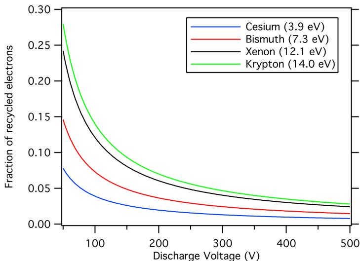
**Figure 3.** The necessary fraction of current from recycled electrons collected at the anode for ionization occurring solely through recycled electrons
