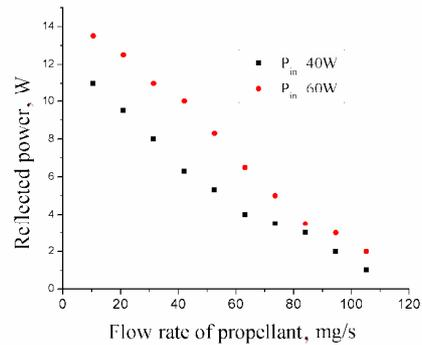
Figure 4. Reflected power vs. Ar mass flow rate
