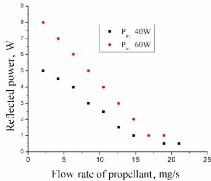
Figure 3. Reflected power vs. He mass flow rate
