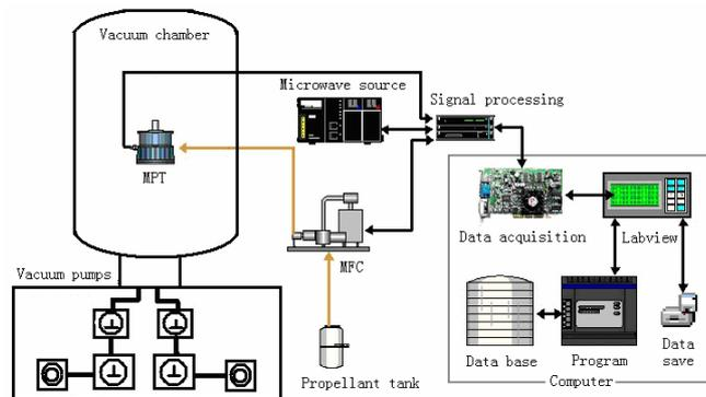
Figure 1. Schematics of MPT vacuum experimental system
