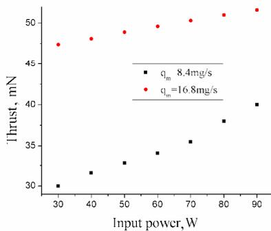
Figure 7. He thrust vs. input power
