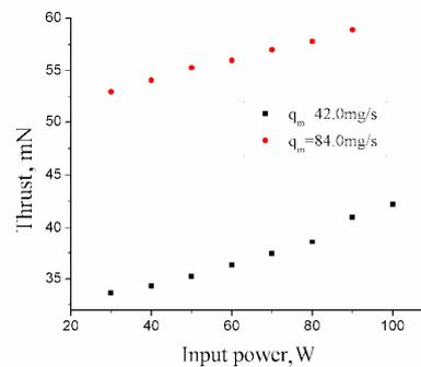
Figure 8. Ar thrust vs. input power
