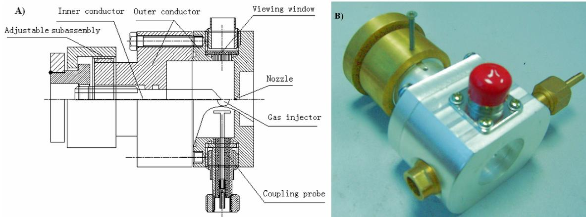
Figure 2. A) Coaxial resonant cavity structure of 100W MPT and B) the photograph of 100W MPT
