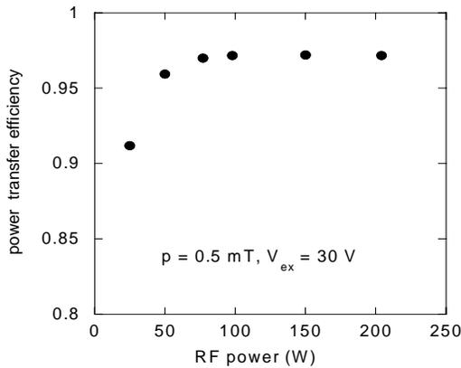
**Figure 2. Power transfer efficiency versus RF power.**
