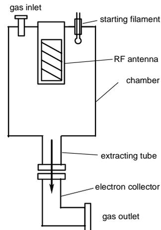
**Figure 1. Schematic diagram of the plasma cathode.**
