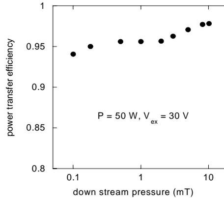
**Figure 3. Power transfer efficiency versus downstream pressure.**
