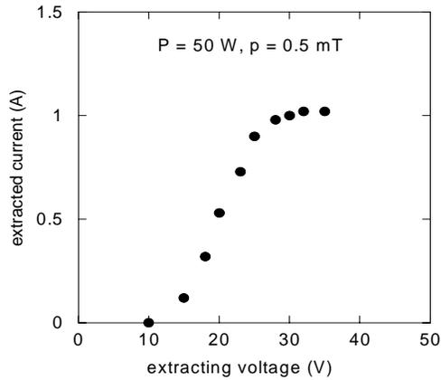
**Figure 6. Extracted electron current versus extracting voltage.**
