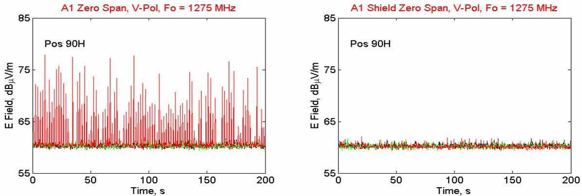
**Figure 10. One hundred zero span pulses taken at postion 90H, at 1275 MHz a) Unshielded PPT, b) Shielded PPT**
