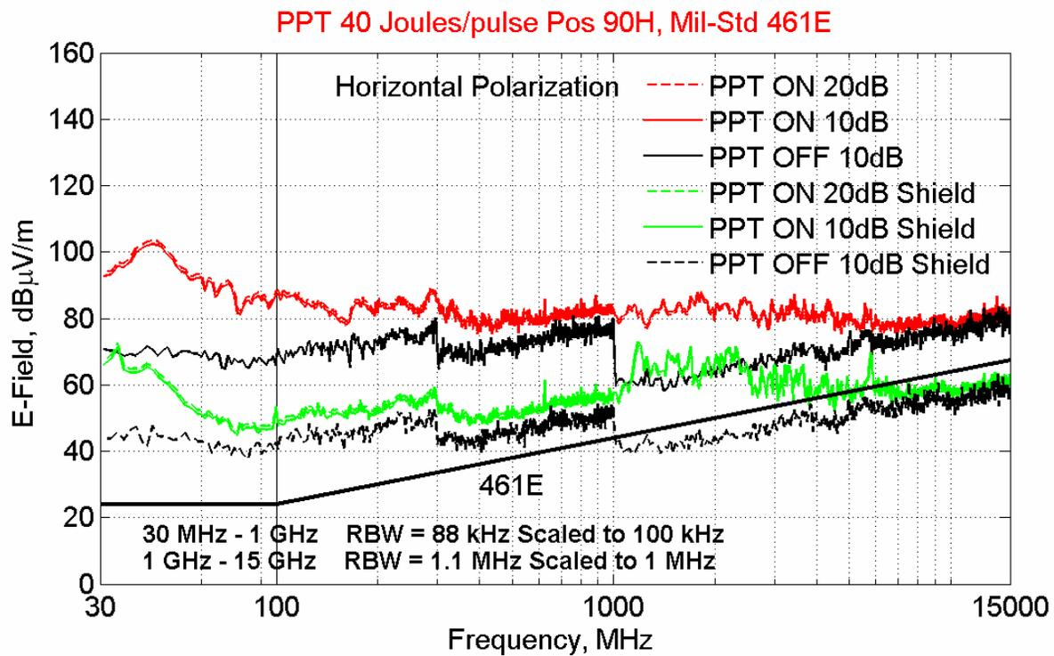
Figure 9. PPT spectral emissions scaled to Mil-STD 461E RBWs, position 90H a) Vertical polarization b) Horizontal polarization
