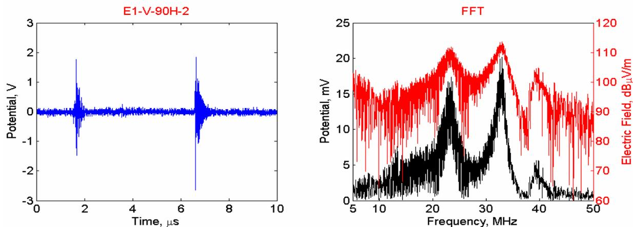
**Figure 6. Typical PPT pulse: a) shows the observed time domain pulse, while b) shows the transformed frequency spectrum. The upper data correspond to the right vertical axis, while the lower data correspond to the left vertical axis.**
