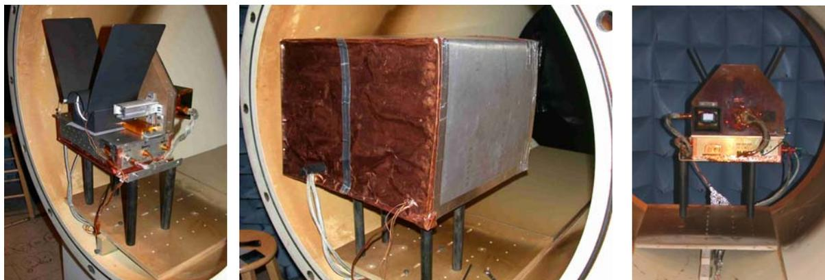
**Figure 5. PPT in dielectric tank: a) unshielded configuration; b) shielded configuration; c) PPT front side viewed from main vacuum chamber**
