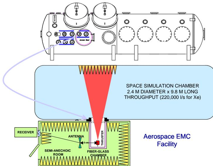
**Figure 1. Layout of the facility used to measure electromagnetic emissions from PPT**
