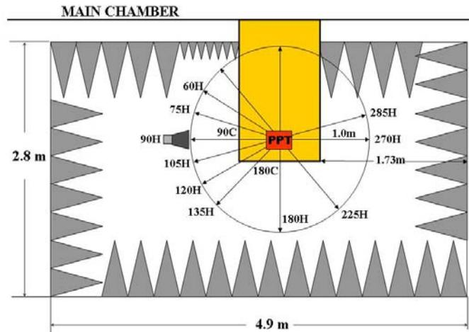
Figure 2. Scale drawing of anechoic room showing antenna and thruster placement
