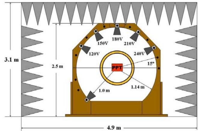
Figure 3. Vertical test configuration showing antenna and thruster positions.
