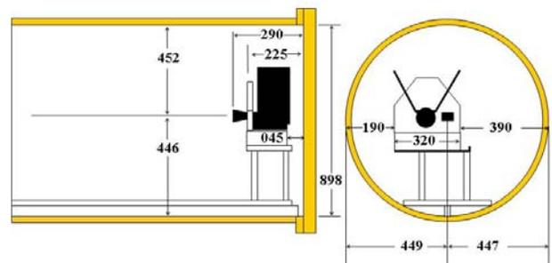
Figure 4. Diagram of PPT in dielectric tank. All dimensions in mm.
