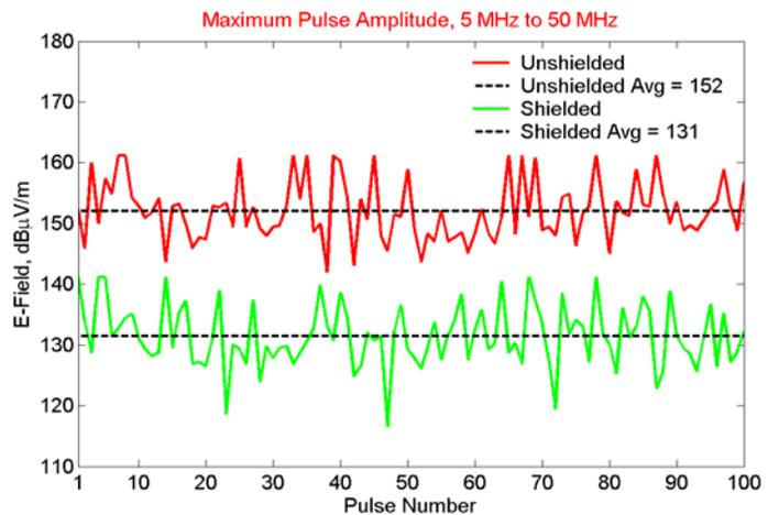
**Figure 7. Maximum pulse amplitude from time domain pulse, in shielded and unshielded configurations**
