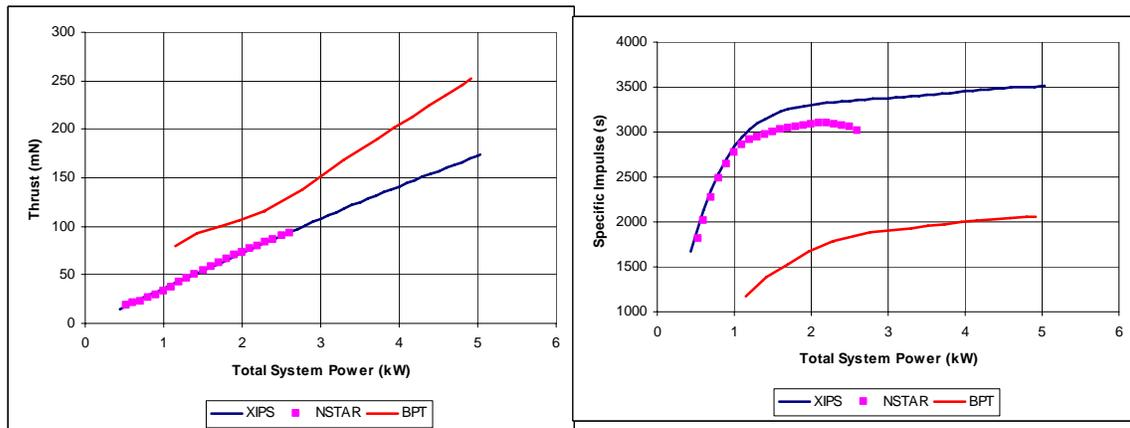
Figure 5: 25 cm XIPS, NSTAR, and BPT-4000 thrust and specific impulse versus PPU input power.
