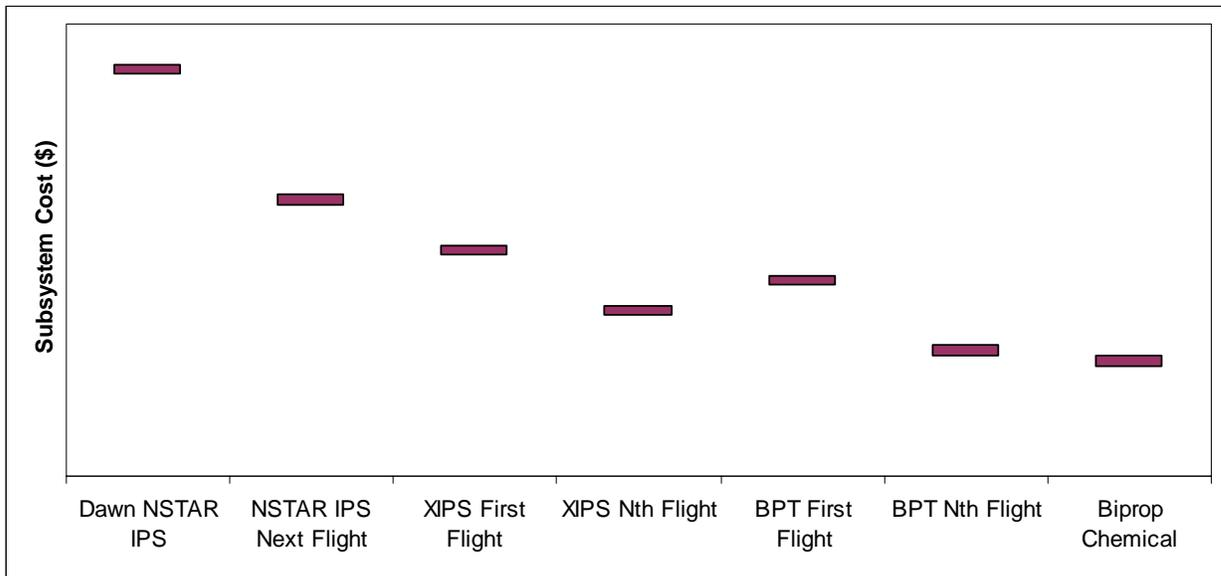
**Figure 14: Cost Comparison of NSTAR, XIPS, BPT, and Chemical propulsion systems (Note: this chart does not include the cost of the solar array)**
