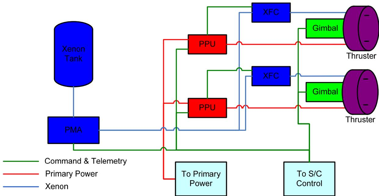
**Figure 3. Solar Electric Propulsion System (SEP) block diagram.**
