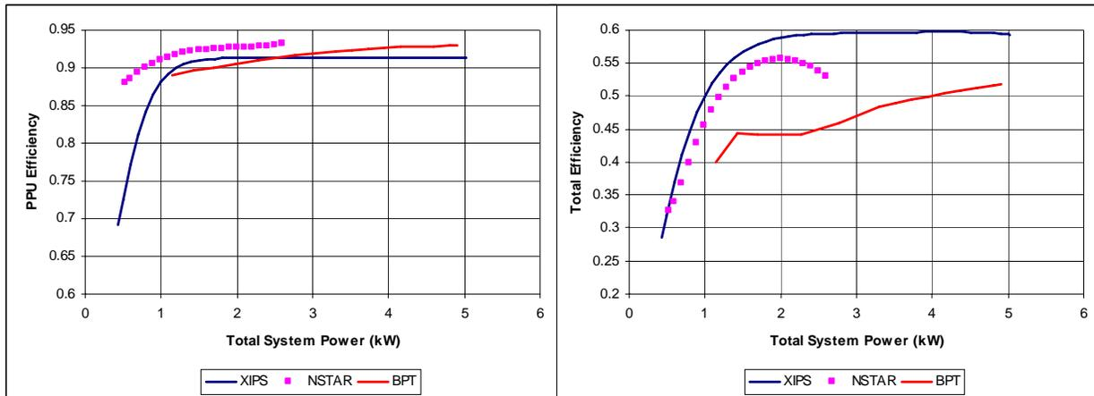
**Figure 7. 25 cm XIPS, NSTAR, and BPT-4000 PPU and total system efficiency versus PPU input power.**
