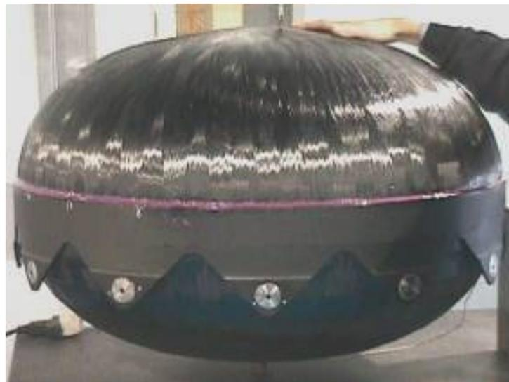
**Figure 9. Dawn xenon propellant tank manufactured by Carleton Technologies.**
