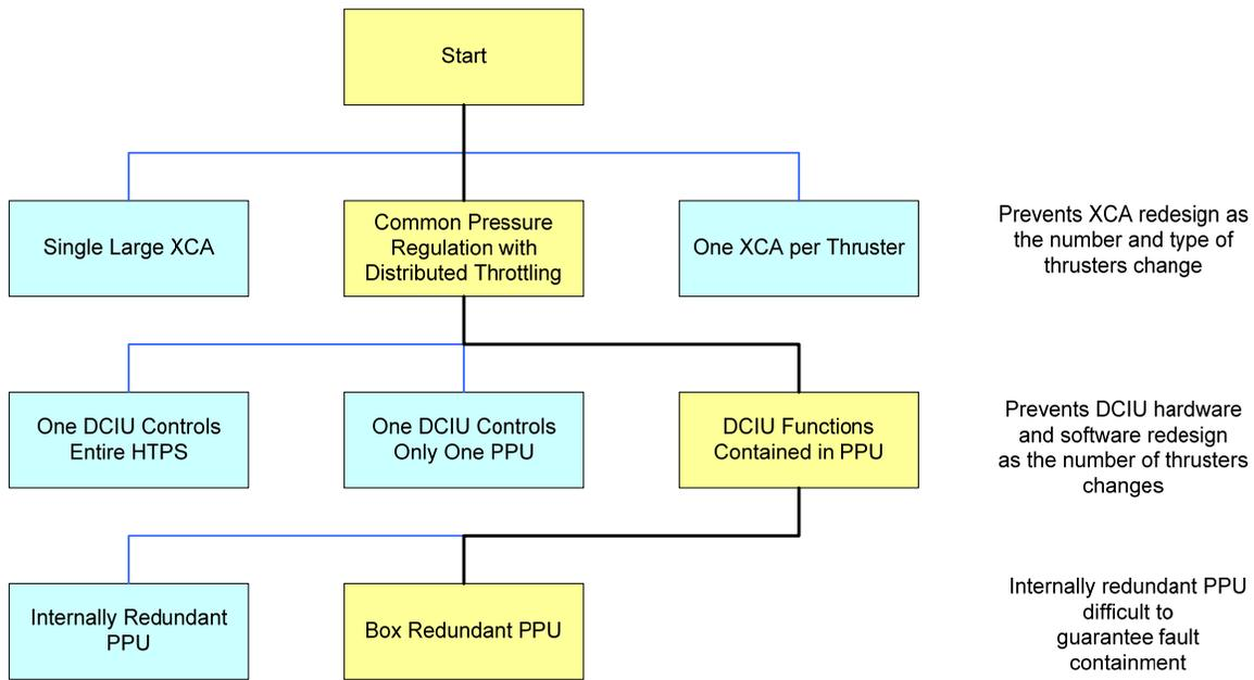
**Figure 2. Solar Electric Propulsion (SEP) standard architecture trade studies.**
