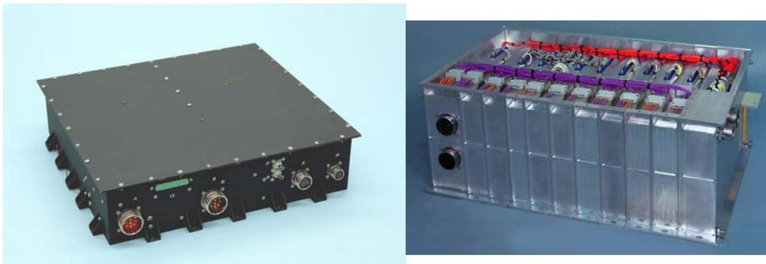
**Figure 6. Aerojet BPT-4000 PPU (left), L-3 25 cm XIPS XPC (right)**
