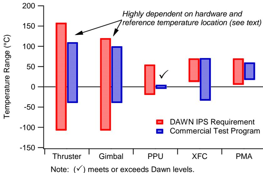
**Figure 11. Temperature range requirements for Hall thruster subsystem components**
