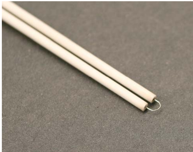
Figure 6. Close up of an emissive probe tip.
